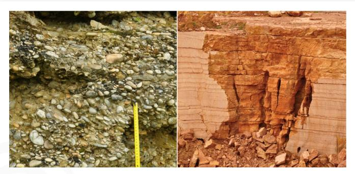
Left: Example of a clastic rock with intergranular porosity; Right: Example of a carbonate rock with fissured porosity
