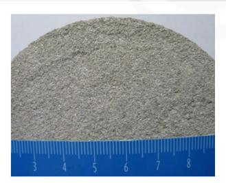
Core of a porous Upper Pannonian siliciclastic reservoir in Slovenia, from a depth of 1.4 km
