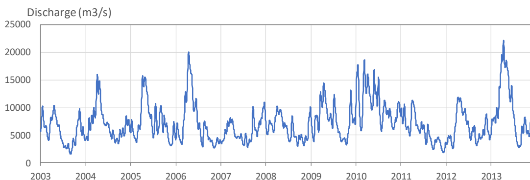
Figure 7.3: Simulated Danube River discharge just upstream of the Danube Delta during the period 2003-2013.
