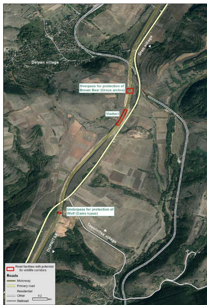
Fig 3. Key defragmentation facilities of the Struma Motorway with the conflicting 1st class road and railroad. (© BBF).
