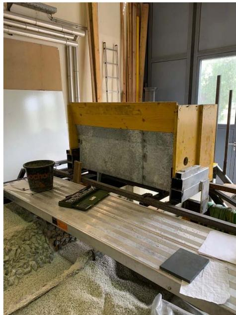
*Figure 27. Sediment feeder at the inlet of the model section.*
