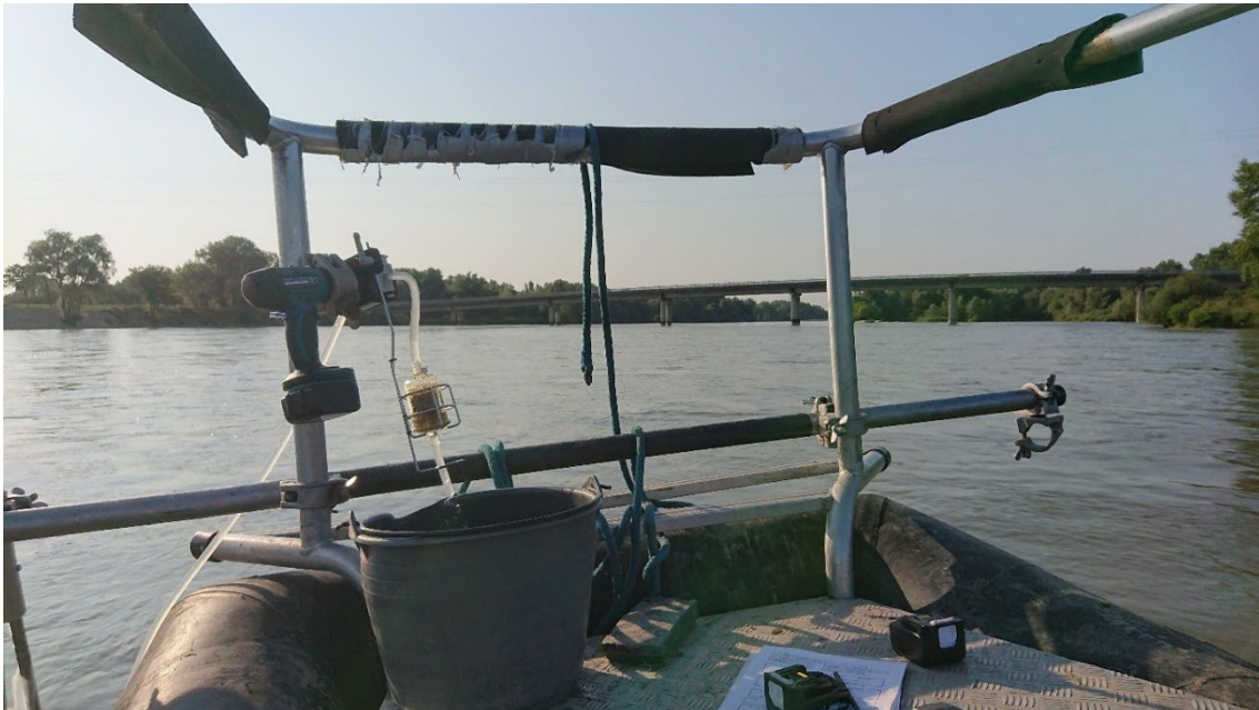
Figure 7: eDNA sampling in the Drava. Water is filtered through the tubes using the pump mounted on the driver-drill. The filter (above the bucket) collects the genetic material.
