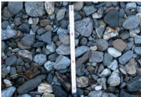
Fig. 23: Grain size is a decisive factor for bedload transport
