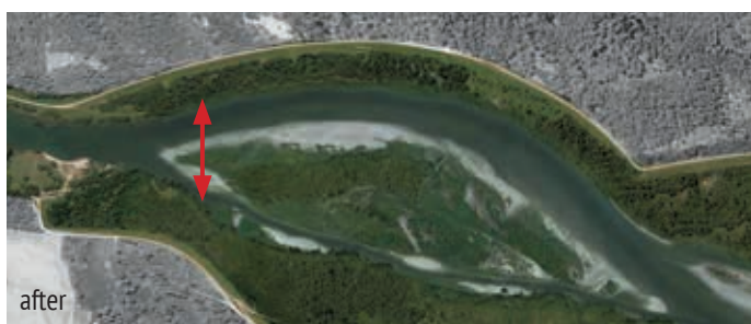
Fig. 48: Combining mechanical widening and the initial channel to replace existing ramps (photo montage; Licca liber, Augsburg, Germany)
