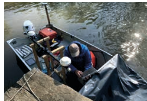
Fig. 25: Boat equipped with modern sonar and laser technology for measuring the bed of Mura
