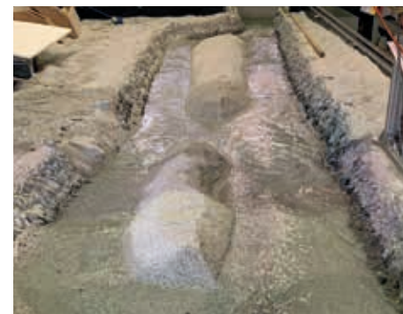
Fig. 27: Physical model for Mura River widening at Gosdorf (Styria, A)
