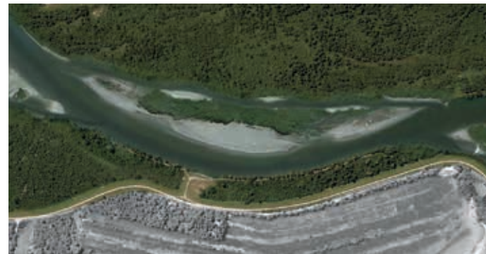
Fig. 68: Combining the lowering of the foreland with an initial channel (photo montage; Licca liber, Augsburg, Germany)
