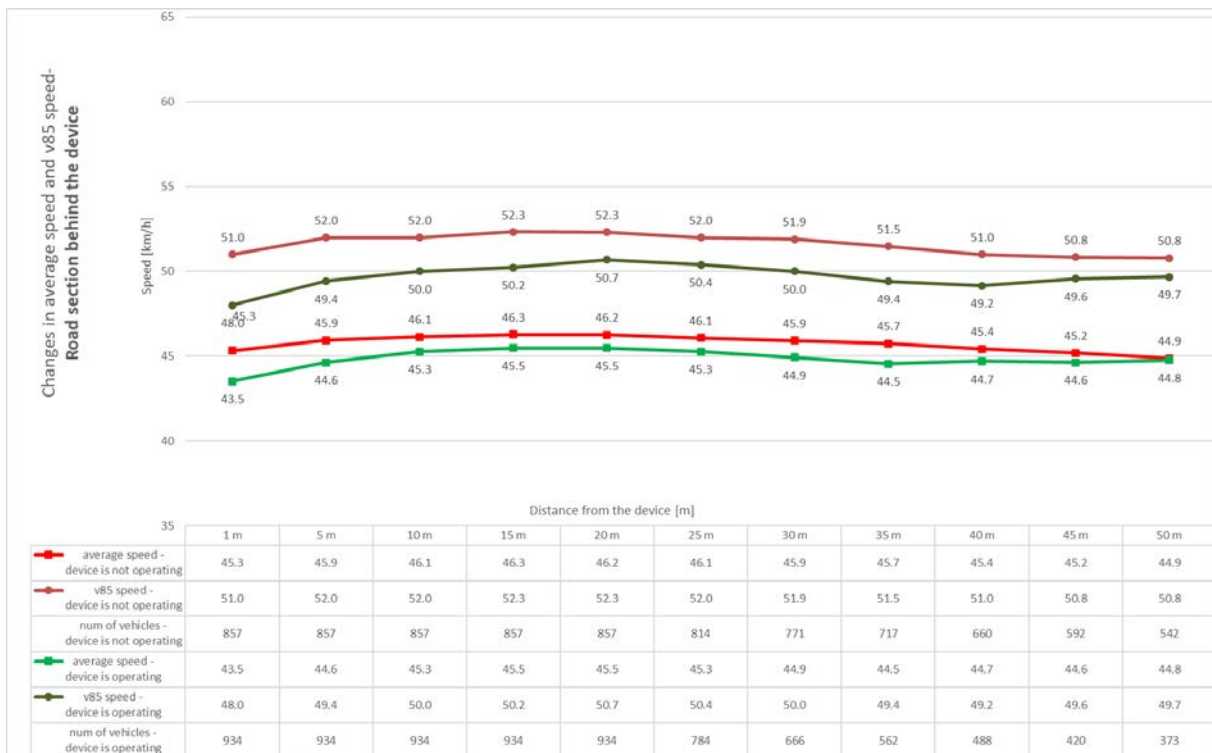
Figure 12: Average and v85 speeds in front of/behind the device- Budapest, Határ road
