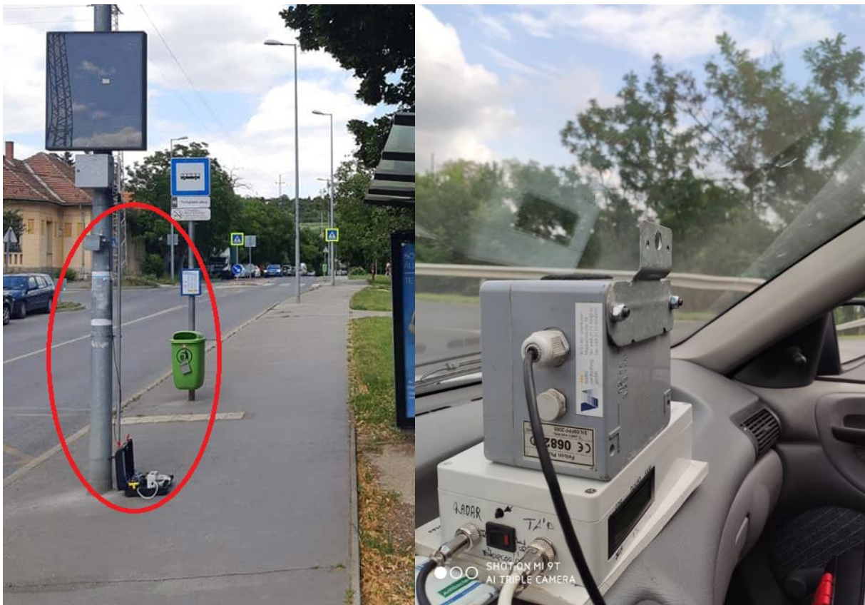
Figure 8: The measuring equipment - Falcon Plus II intelligent microwave detector
