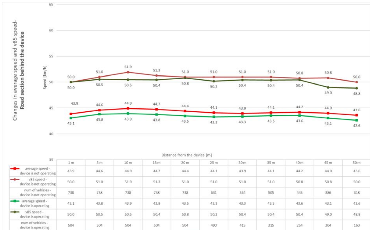
Figure 14: Average and v85 speeds in front of/behind the device- Budapest, Ezüsthely street
