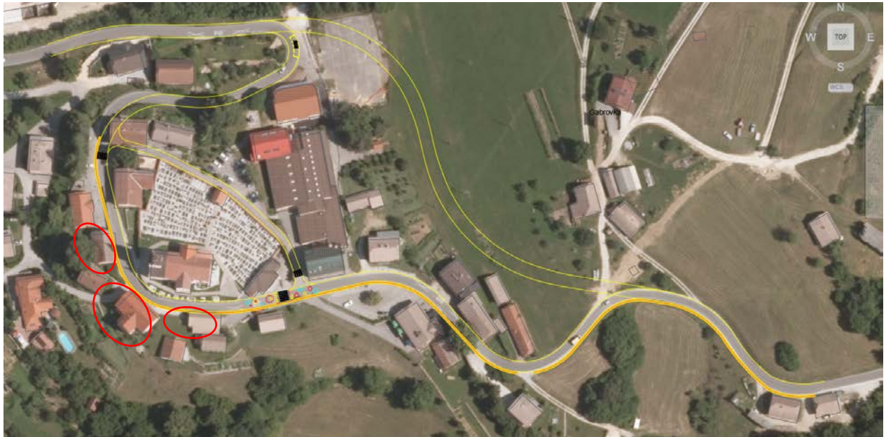
Figure 56 Proposed alignment of sidewalk in Gabrovka (1.20 m width, 450 m long)
