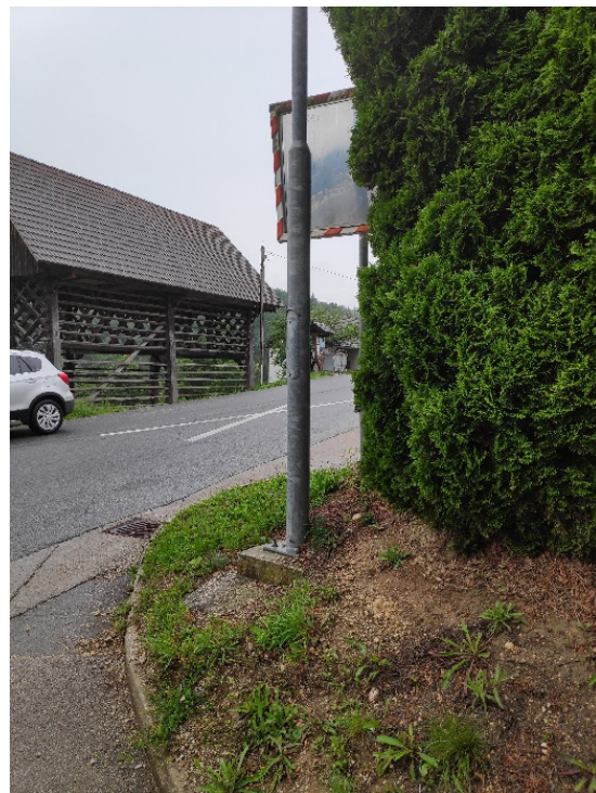
Figure 51 Entrance to the school parking place – poor sight distance on the right-hand side at Location 1
