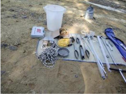
Sediment core samplers for shallow sediments and bank soil
