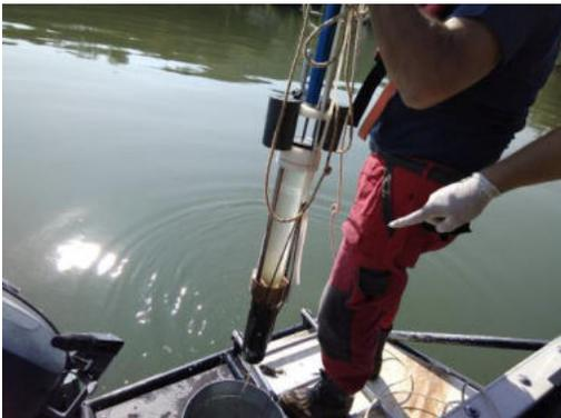
Undisturbed sediment core sampler
