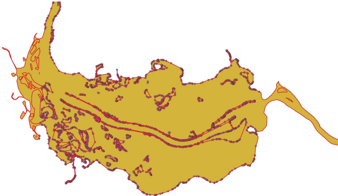
Figure 11: Parts of the newly created polygon in brown (“AT_DU_AFP_PG”), the inundation areas in a polyline format (red lines) and the points of the first suggested floodplain (“Floodplain_0”) are shown.
