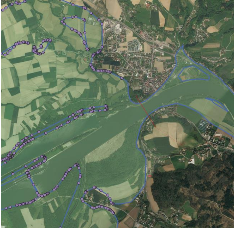
Figure 13: End (red line) of the first floodplain in Austria. Blue lines show the inundation area as polylines. Purple points show the “Floodplain_0” layer.
