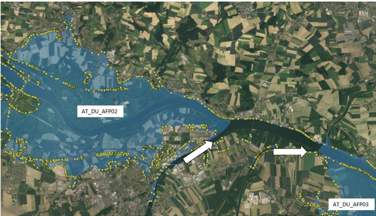
Figure 17: Hydraulically active floodplains (AT_DU_AFP02; AT_DU_AFP03) along the Austrian Danube separated due to the confluences of tributaries (white arrows).
