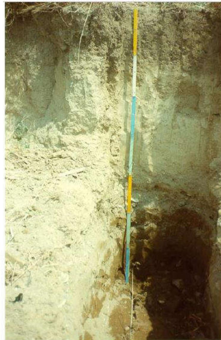
Fig. 12. Floodplain sediment sequence with soil development in Greece. Meter: coloured sections 20 cm. Fine-grained clay and silt down to a depth of 75 cm (low energy floodplain sediment - good for sampling, soil has developed down to a depth of 25-29 cm). Coarse-grained sandy and pebbly unit between 75-100 cm (high energy environment). Sandy-clay unit between 100-134 cm (low-energy environment). Gravel bed below a depth of 134 cm. Photo: A. Demetriades, IGME.
