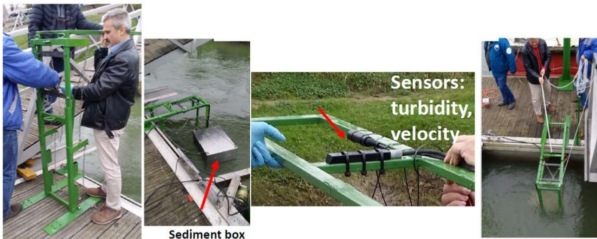
**Figure 5.** The installation of the JDS sediment trap box into the river requires a manually operated fix crane. The Velocity and turbidity sensors data is used to estimate the sediment and water quantity that reached the sediment trap during the collection period.
