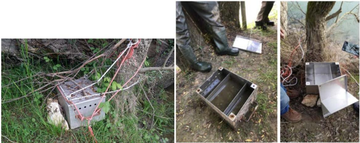
**Figure 9.** Left: standard sediment trap box emplaced on the floodplain. Right: suspended sediment trapped by the box during the last flooding event.
