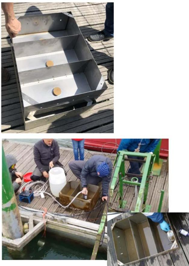
**Figure 7.** *The standard JDS has been converted to the tool applicable for regular monitoring sample collection. The holes-and-plugs innovative development has reduced the sample removal from 1 hour (see picture on the right) to 20 minutes (see the picture on the left).*
