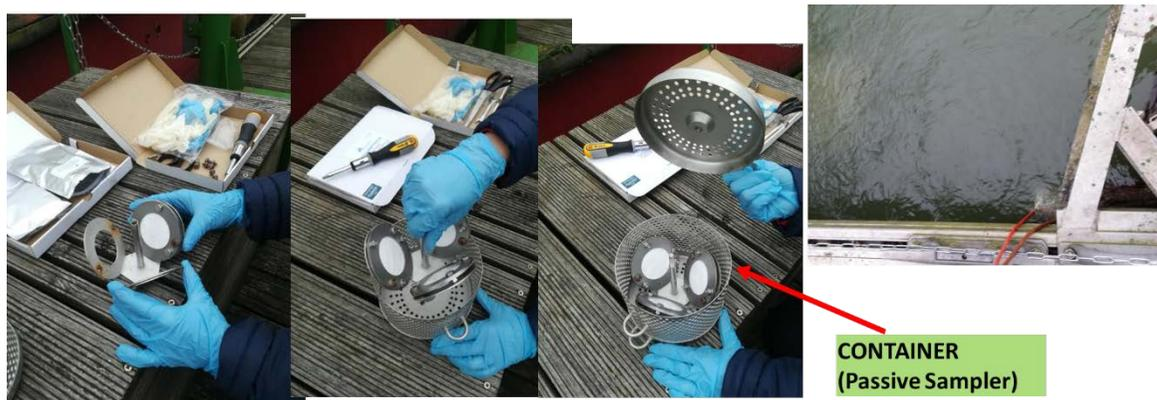
**Figure 4.** *The passive membrane sampler ('artificial fish'). Note the 3 different types of selective sampling membranes: Pesticides, PAHs and Metals.*
