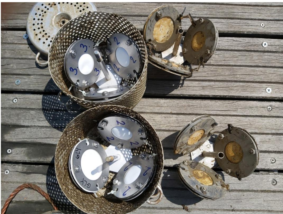
**Figure 15.** *Passive samplers before and after one month use in the Drava River.*
