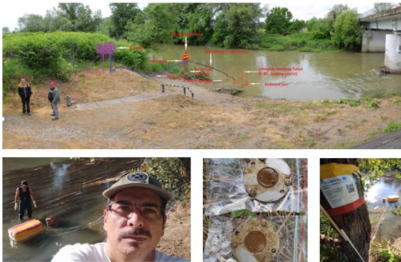
**Figure 10.** Standard JDS sediment trap box and passive membrane installed in the Upper Tisa Test Area, Romania. The JDS box originally developed for large rivers has been adapted to suspended sediment sampling in shallow river by the SIMONA project.
