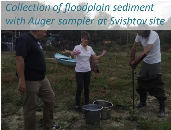
*Collection of floodplain sediment with Auger sampler at Svishtov site*
