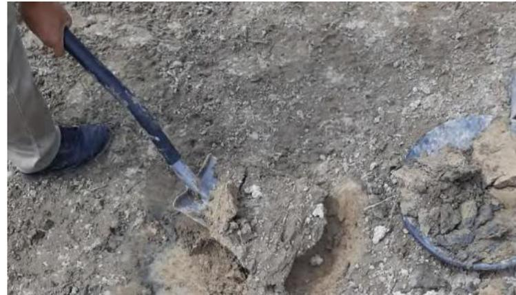
*Topsoil of the floodplain sediments at Pristol (sampling depth: 0-5 cm)(left); Hole dug for bottom soil sampling at 40-50 cm depth (right)*
