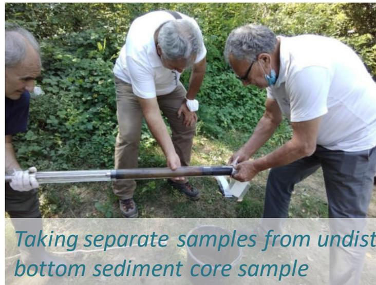
*Taking separate samples from undisturbed bottom sediment core sample*
