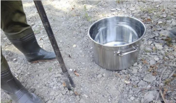
*Collection of floodplain sediment with Auger sampler at Iskar R. site*
