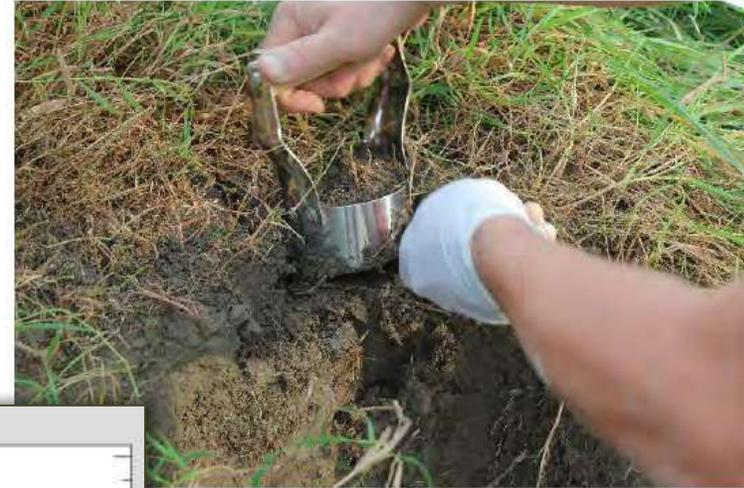
extracting top soil from floodplain sediment using the cake sampler
