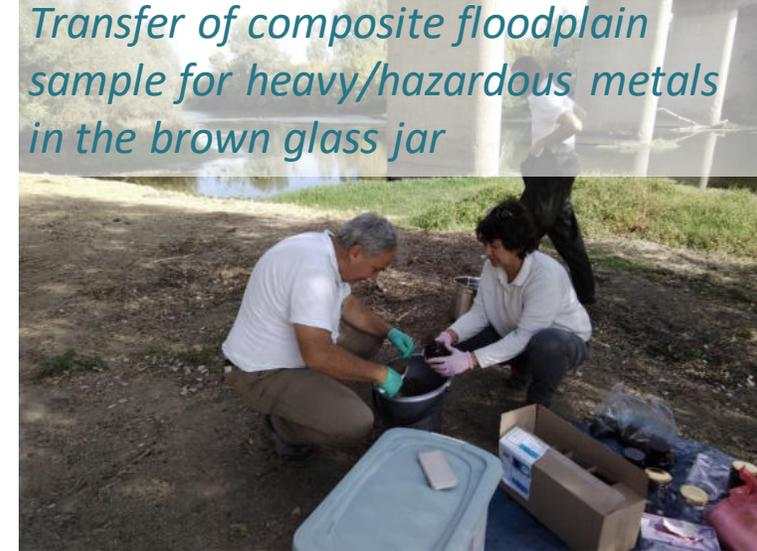
*Transfer of composite floodplain sample for heavy/hazardous metals in the brown glass jar*
