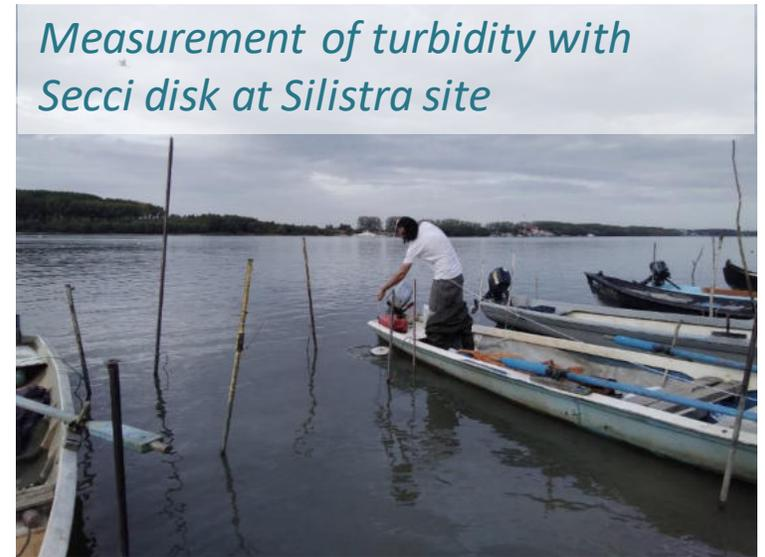
*Measurement of turbidity with Secci disk at Silistra site*
