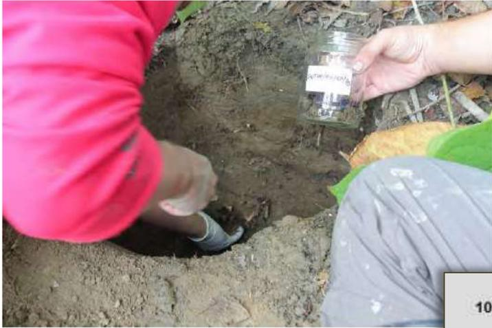
Figure 4.5. Loading jar with floodplain sediment (bottom layer)
