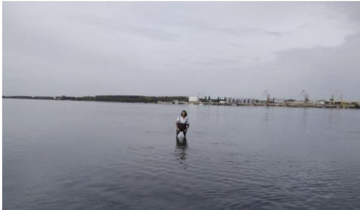
*Collection of suspended sediment with plastic can at Svishtov site*
