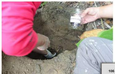
Figure 4.5. Loading jar with floodplain sediment (bottom layer)
