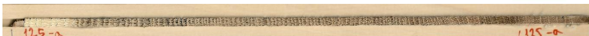
Figure 4. A sample of prepared and scanned pedunculate oak core for measuring tree-ring width.
