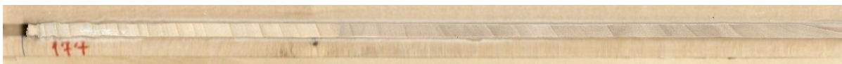
Figure 1. A sample of prepared and scanned core of Euroamerican poplar for measuring the tree-rings width.
