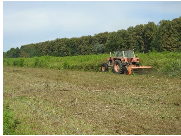
Figure 5: Claas Celtis 90KS, mulcher: Berti TSB 230.
