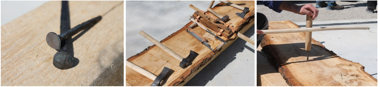
Photos by Miriam Sapio from left to right: Hand-forged Roman nails, a sortiment of reconstructed Roman tools, a Roman bow drill in action.
