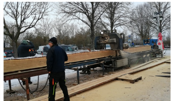
Photo right: The mobile sawmill from Bremen was able to saw excess lengths of up to 19.30 m, which was necessary due to the continuous planks of the boat (Photo by Margit Schedel).
