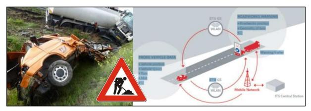
As far as work-zone safety is concerned, there are additional pilots and tests being implemented in the field of Road works warning (RWW) information generation and distribution. A set of warning message signs are not only shown on VMS facilities but also transmitted into a vehicle's OBU.
