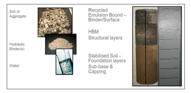
Besides its technological/functional characteristics, further advantage and benefits of HBM technology clearly lies in its ecological aspects, when the waste material from re-surfacing can again be used for the new surface layers.
