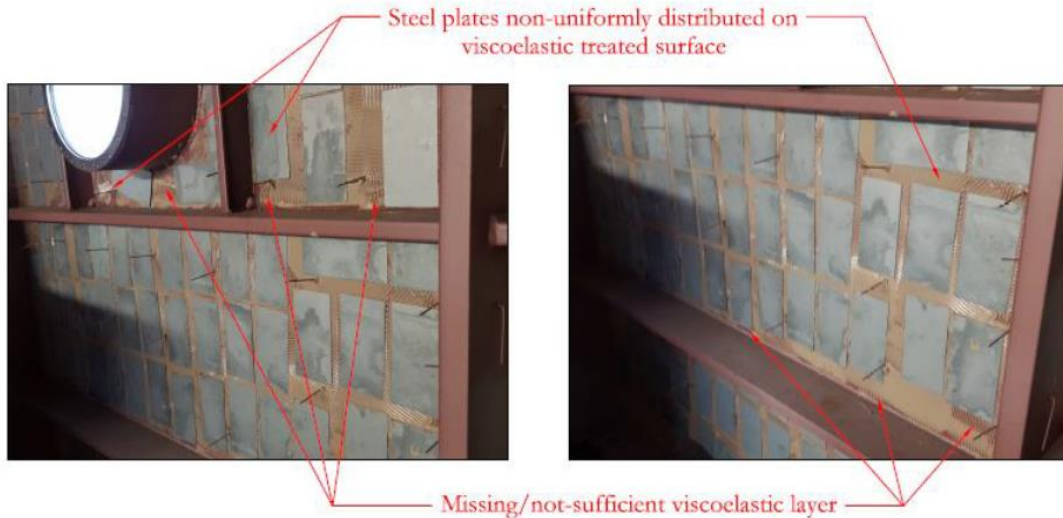
Abstract from developed technical report after survey performed on board, proposals for damping treatment optimization
