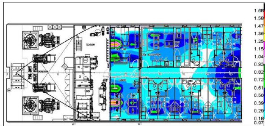
Figure 89 – Calculated vibration level in aft crew accommodation areas
