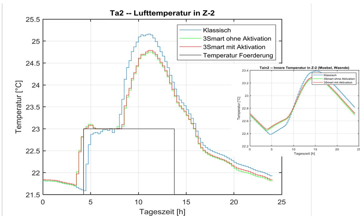
Figure 2.10. Temperature in Z-2. Small figure shows the behaviour of the inner room temperature state (representing walls and furniture).
