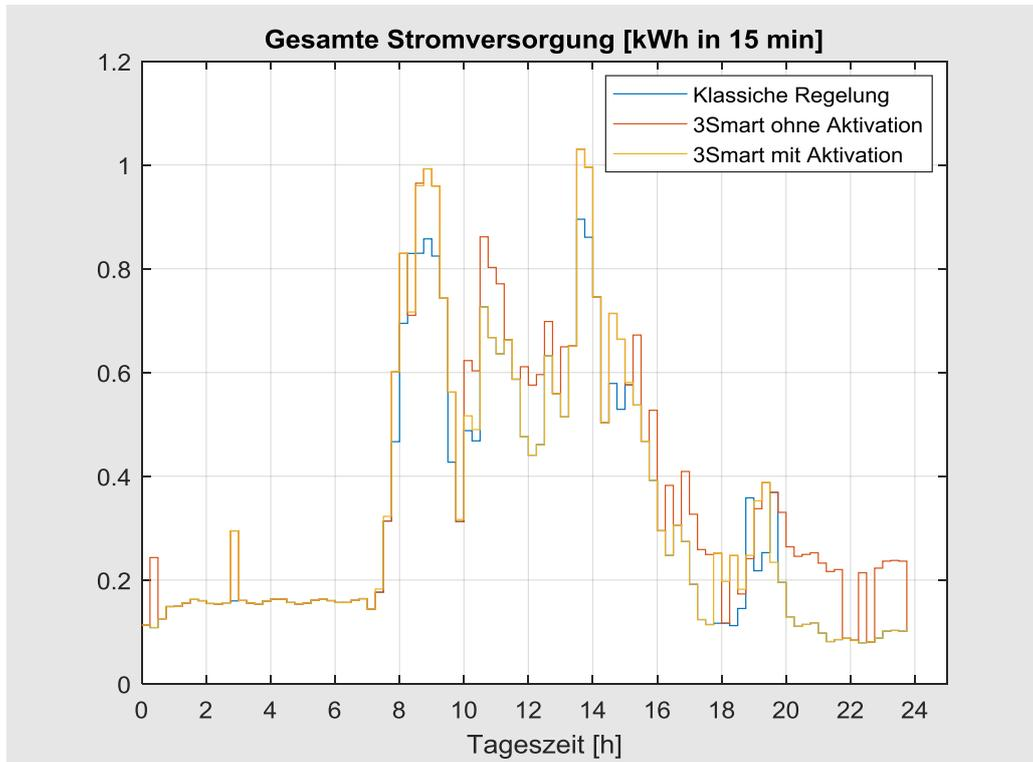
**Figure 2.49.** Overall electricity exchange profile between the building and the grid.
