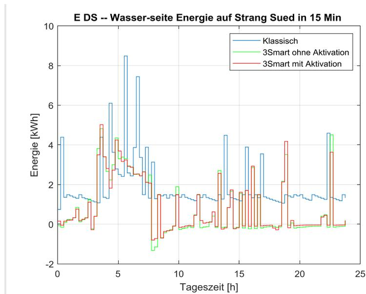
Figure 2.46. Consumed water-side energy on duct south.
