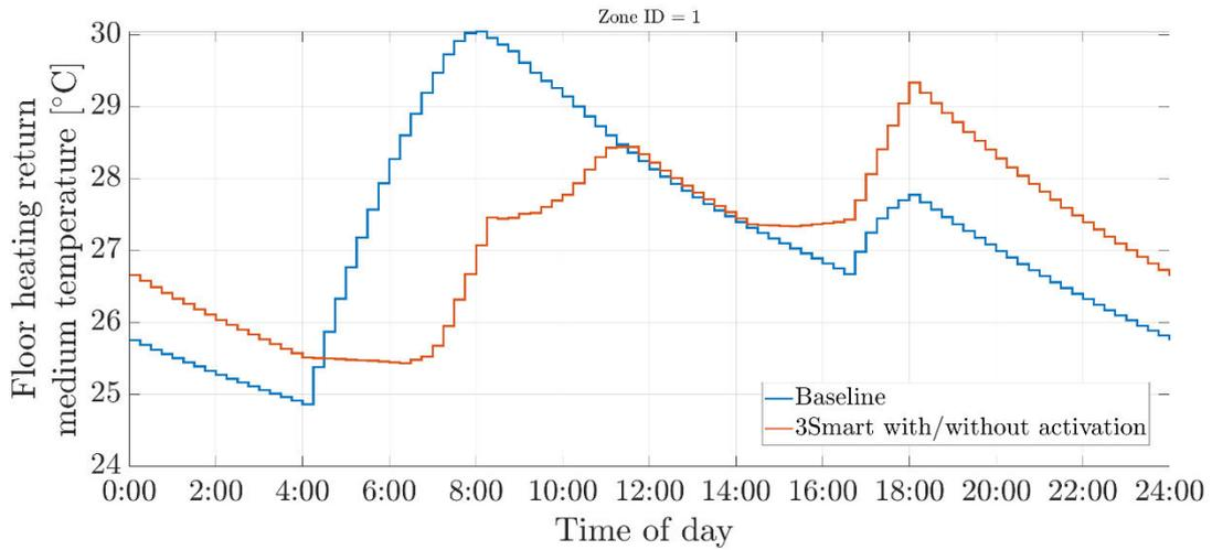
Figure 3.20. Return medium temperature from the floor heating element in the exemplary room in retirement and care centre within the analysed day.
