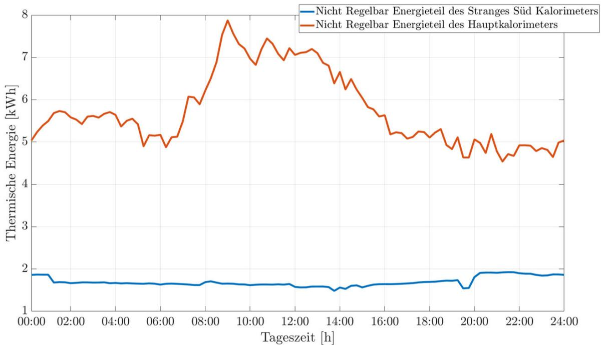
**Figure 3.16.** Non-controllable consumption of thermal energy on the HVAC level, for a sunny workday in November.
