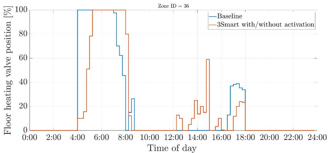
**Figure 3.25.** Opening of the valve of the floor heating element in the retirement and care centre building room within the analysed day.
