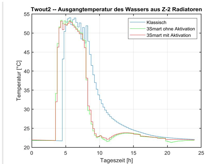
Figure 2.11. Return medium temperature in Z-2.
