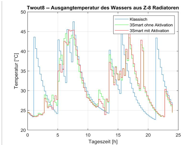
Figure 2.35. Return medium temperature in Z-8.
