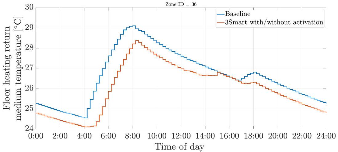
**Figure 3.24.** Return medium temperature from the floor heating element in the retirement and care centre building room within the analysed day.
