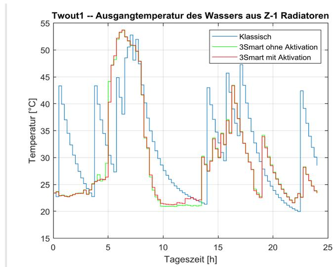
Figure 2.7. Behaviour of the return medium temperature of the radiator in Z-1.
