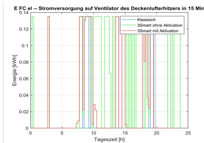
**Figure 2.40.** Electricity consumed on the fan coil in Z-9.
