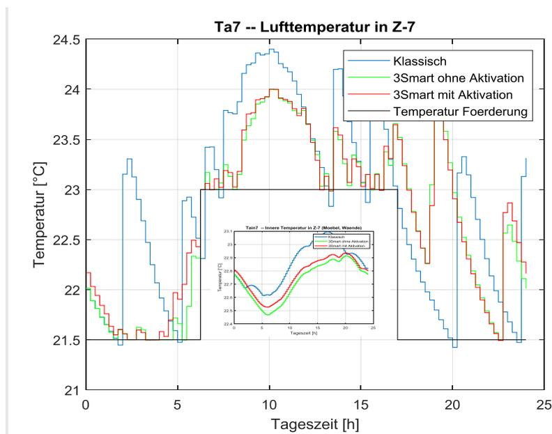
Figure 2.30. Room temperature in Z-7. Small figure shows the behaviour of the inner room temperature state (representing walls and furniture).
