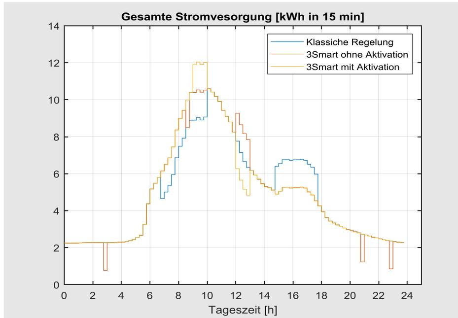
**Figure 3.32.** Overall electricity consumption profile of the retirement and care centre building.
