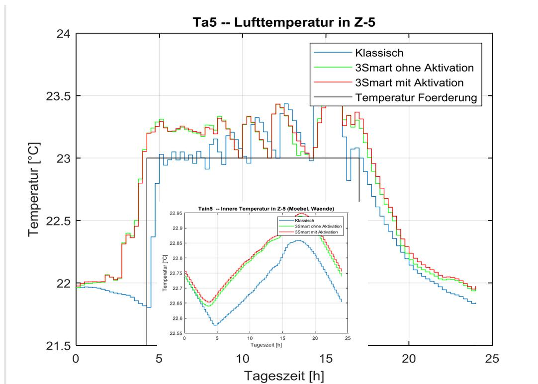
Figure 2.22. Z-5 room temperature behaviour. Small figure shows the behaviour of the inner room temperature state (representing walls and furniture).
