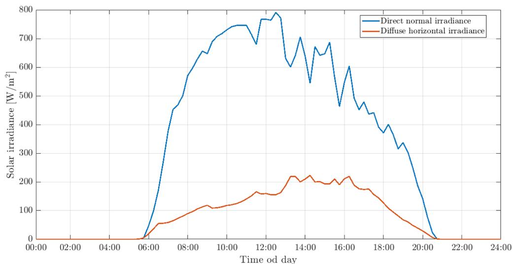
Figure 3.2. Direct (normal) and diffuse (horizontal) solar irradiance for a sunny day in July.
