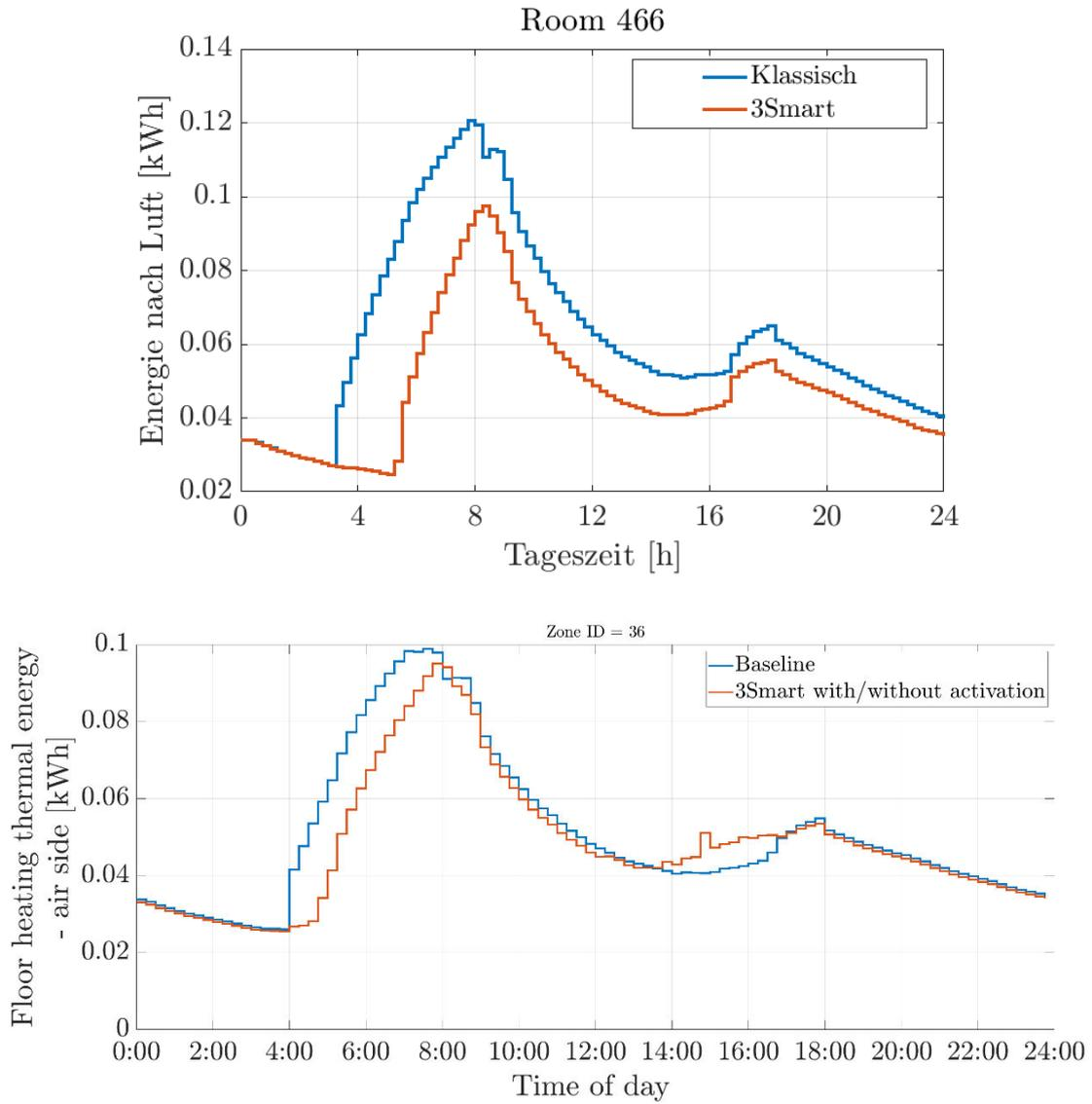
Figure 3.23. Energy provided to air in a room in the retirement and care centre building within the analysed day.
