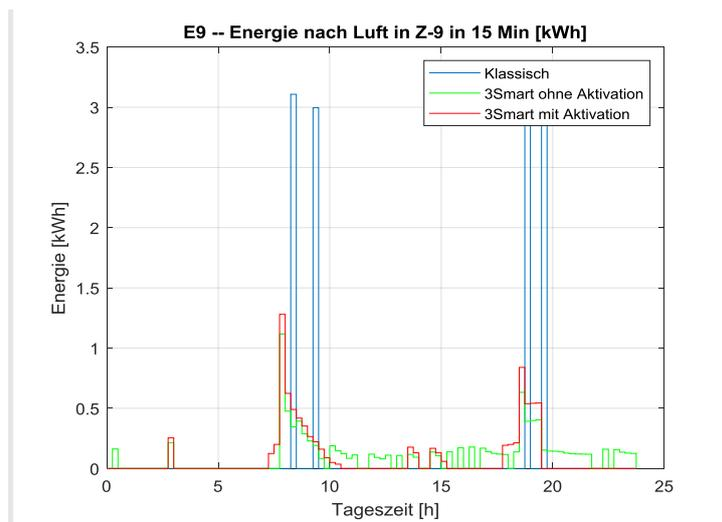
Figure 2.39. Energy provided to room air from the fan coil.
