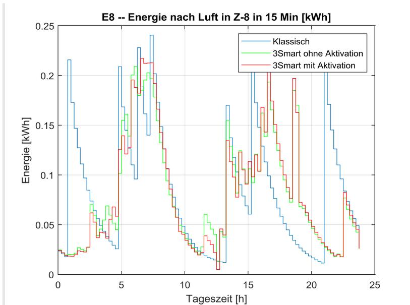
Figure 2.36. Energy provided to room air from radiators in Z-8.
