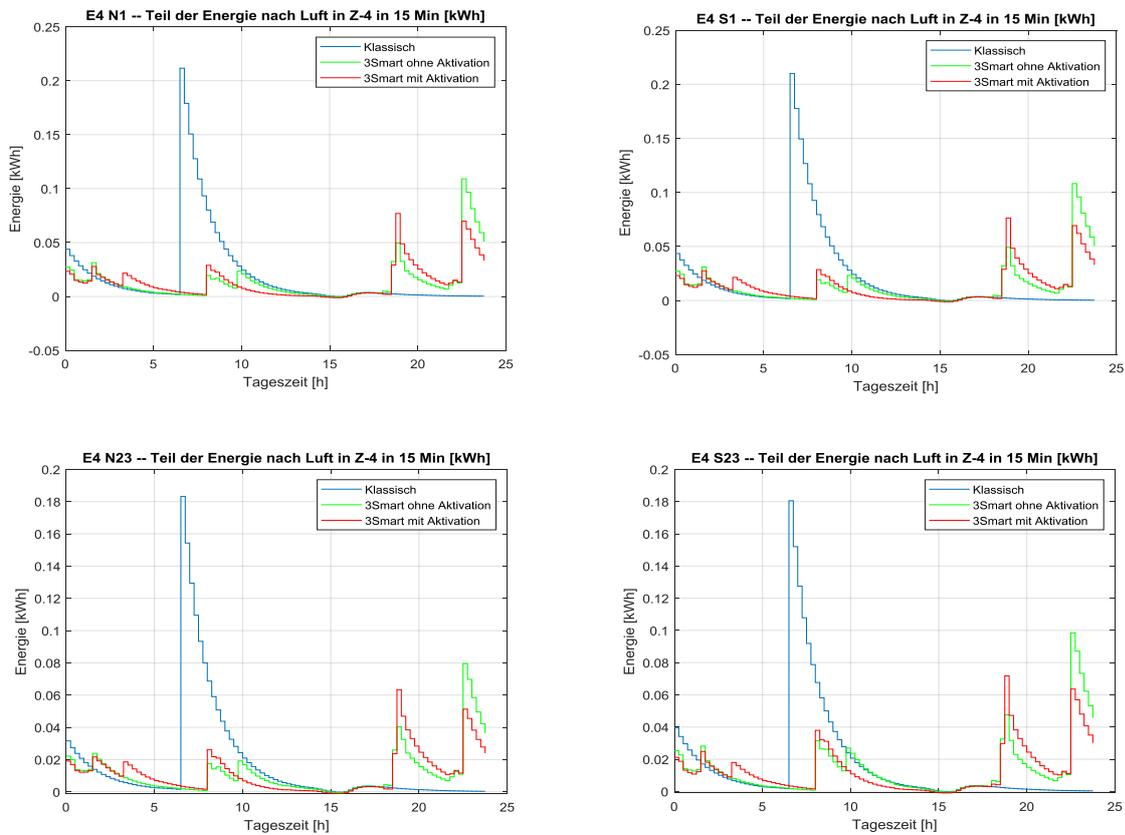
**Figure 2.20.** Energies provided to room air from different radiators groups in Z-4. (left: north duct; right: south duct; up: first radiator on a duct; down: last radiators on a duct).
