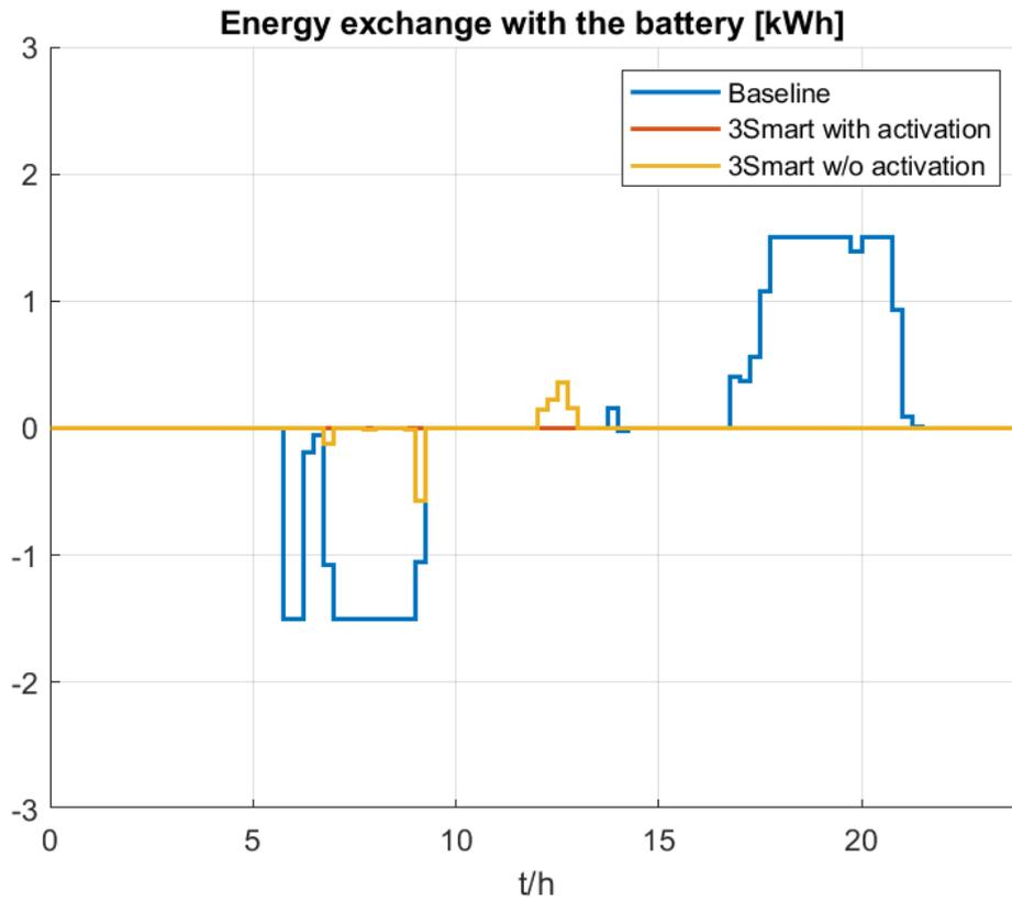
Figure 3.11. Battery charging/discharging energies within the analysed day.
