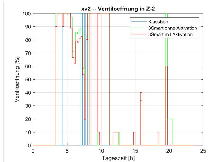
Figure 2.13. Valve opening in Z-2.
