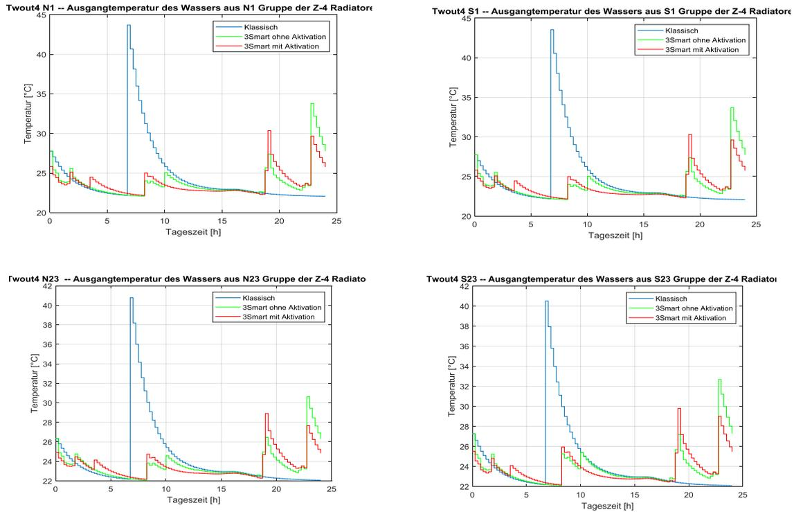
**Figure 2.19.** Return medium temperatures from the four positions of radiators in Z-4 (left: north duct; right: south duct; up: first radiator on a duct; down: last radiators on a duct).
