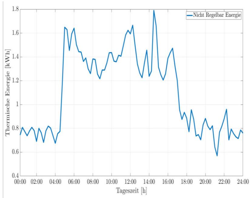
**Figure 2.3.** Non-controllable consumption of thermal energy on the central HVAC system level, for a sunny workday in November.
