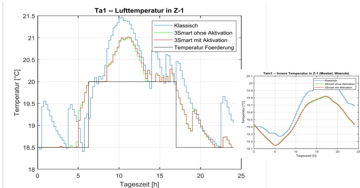
Figure 2.6. Room temperature over time in Z-1 for conventional control and 3Smart strategies. Small figure shows the behaviour of the inner room temperature state (representing walls and furniture).
