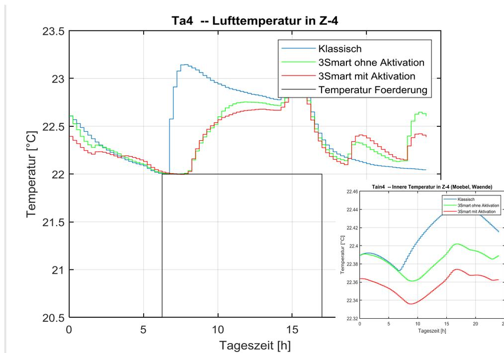
Figure 2.18. Temperature in Z-4. Small figure shows the behaviour of the inner room temperature state (representing walls and furniture).
