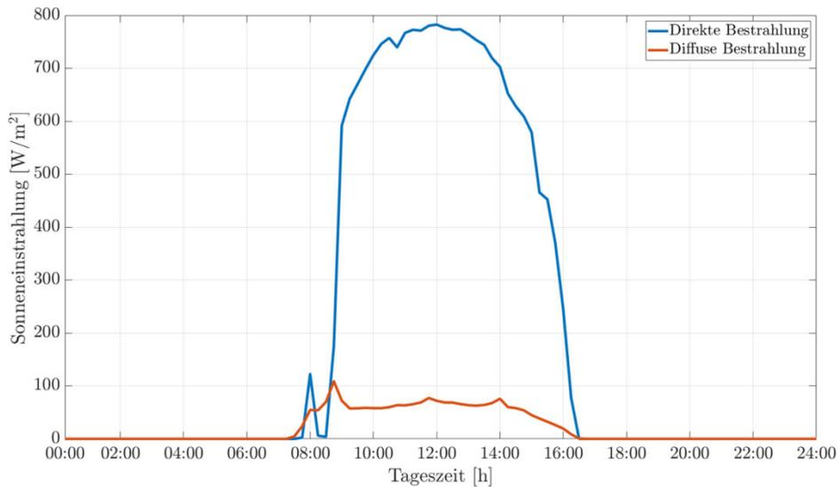
**Figure 3.15.** Direct (normal) and diffuse (horizontal) solar irradiance for a sunny day in November.
