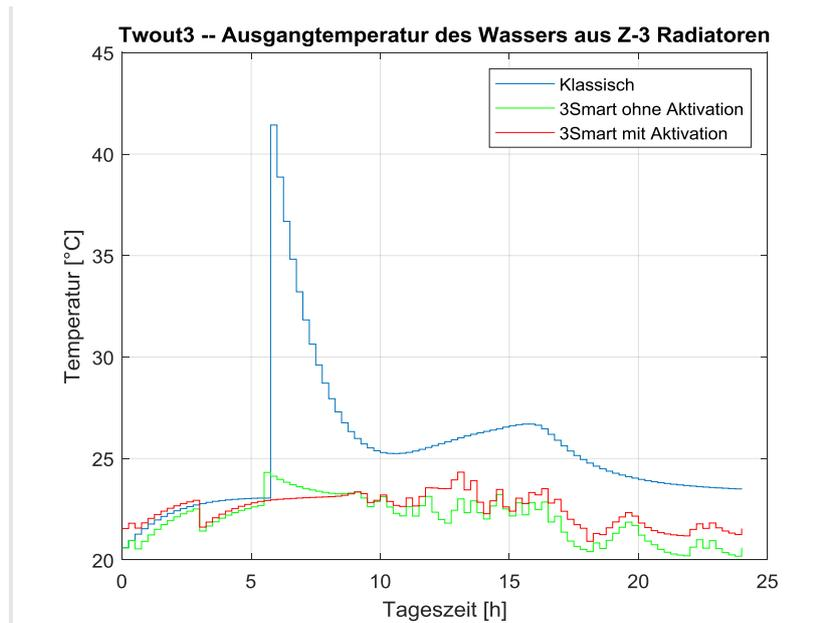
Figure 2.15. Return medium temperature in Z-3.
