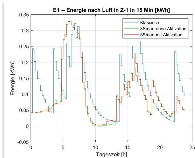
Figure 2.8. 15-minutes energies exerted to room air from the radiator in Z-1.
