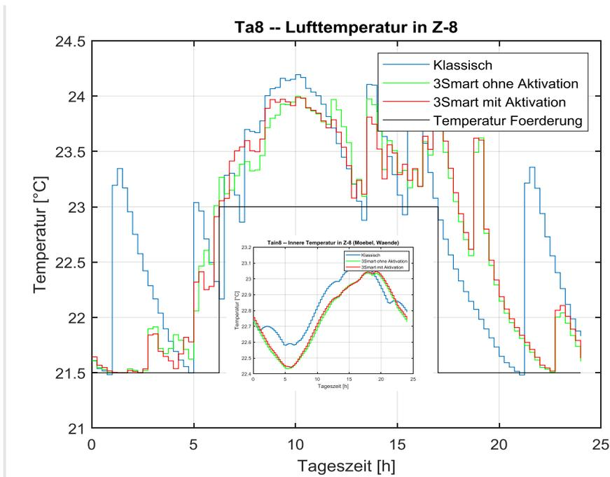
Figure 2.34. Air temperature in Z-8. Small figure shows the behaviour of the inner room temperature state (representing walls and furniture).
