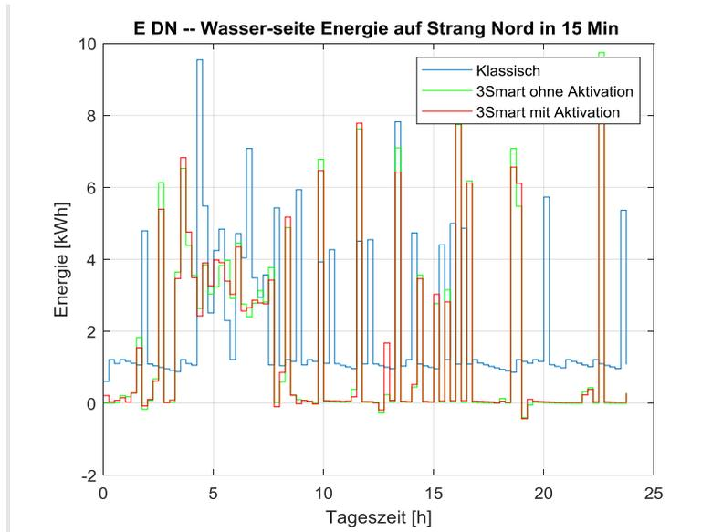
Figure 2.45. Consumed water-side energy on duct north.
