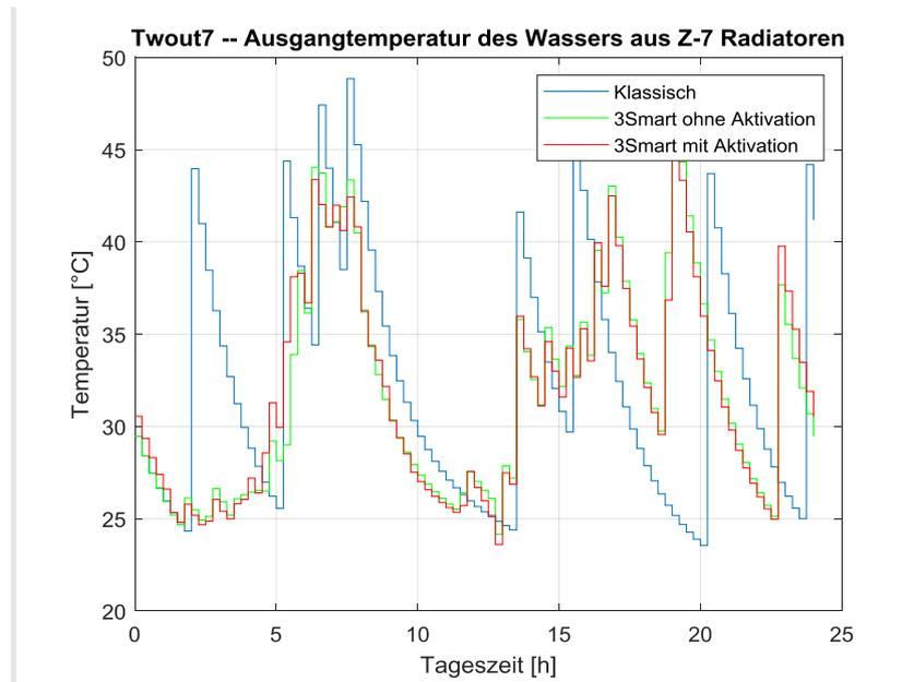
Figure 2.31. Return medium temperature in Z-7.
