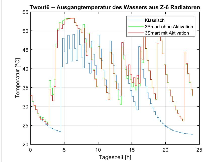
Figure 2.27. Return medium temperature in Z-6.
