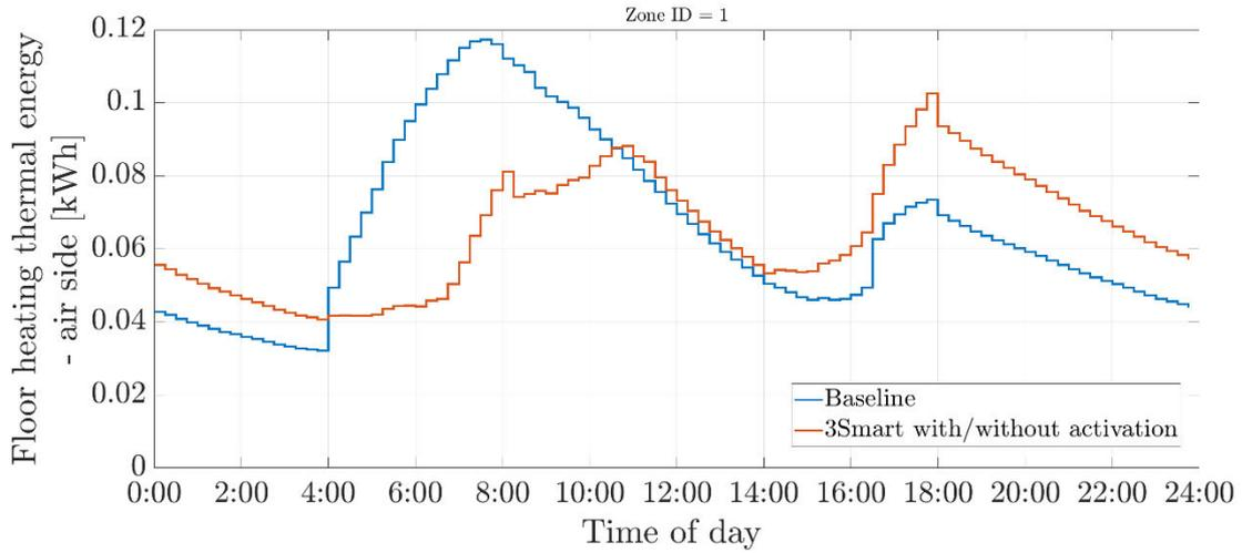
Figure 3.19. Energy provided to air in the retirement and care centre for one exemplary building room within the analysed day.
