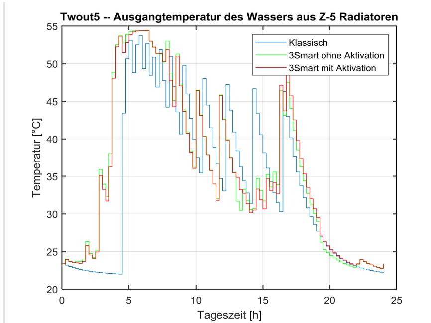
Figure 2.23. Return medium temperature in Z-5.
