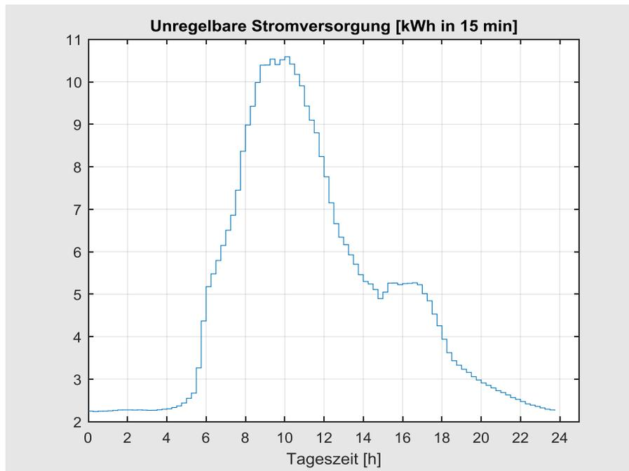
**Figure 3.17.** Non-controllable electrical energy consumption on the microgrid level, for a sunny workday in November.
