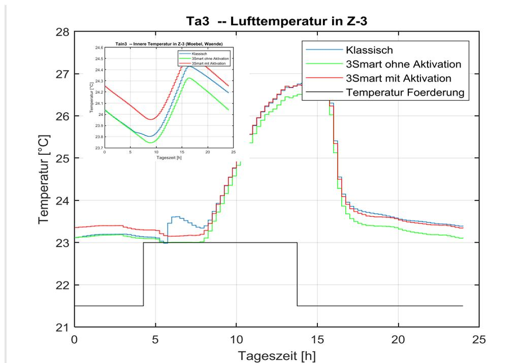
Figure 2.14. Temperature behaviour in Z-3. Small figure shows the behaviour of the inner room temperature state (representing walls and furniture).
