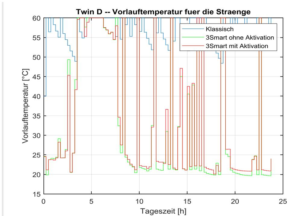
**Figure 2.41.** The commanded starting medium temperatures on the heating substation.
