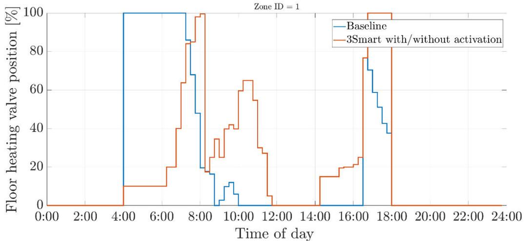
**Figure 3.21.** Opening of the valve of the floor heating element in the exemplary zone in retirement and care centre building within the analysed day.
