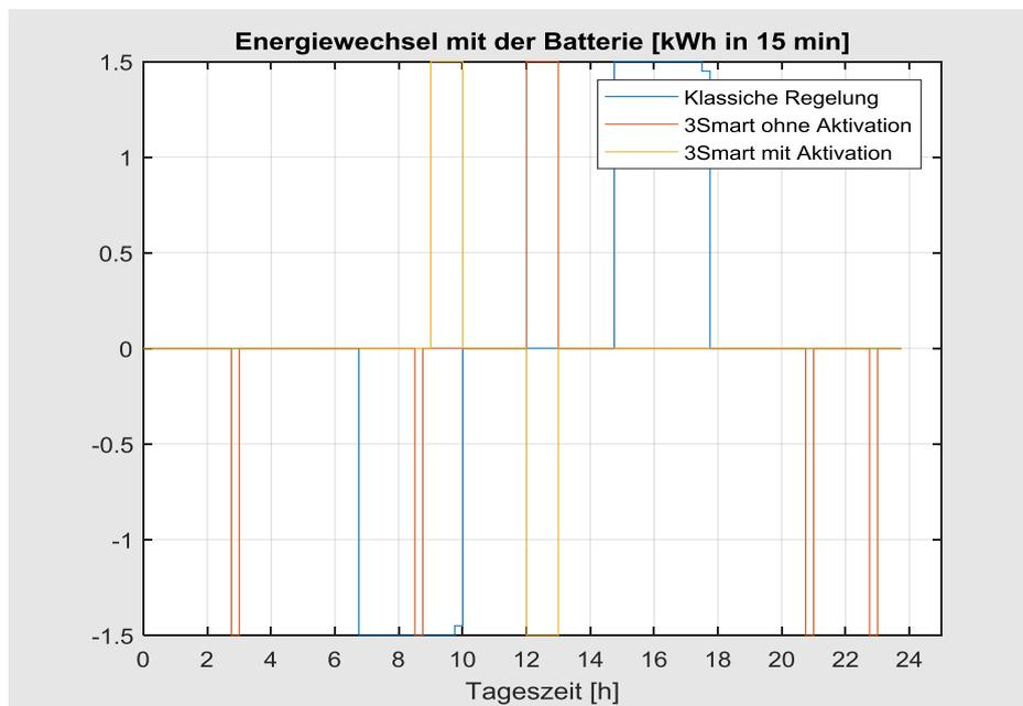
**Figure 3.31.** Battery system actuation on the retirement and care centre building.
