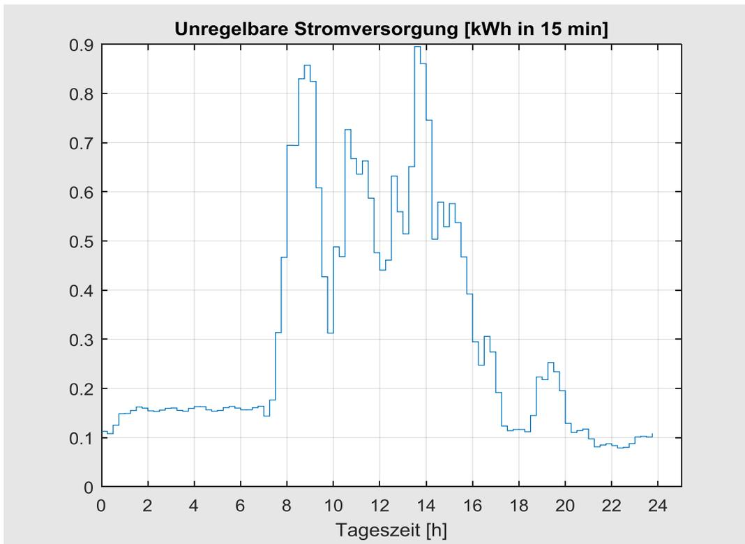
**Figure 2.4.** Non-controllable electrical energy consumption on the microgrid level, for a sunny workday in November.
