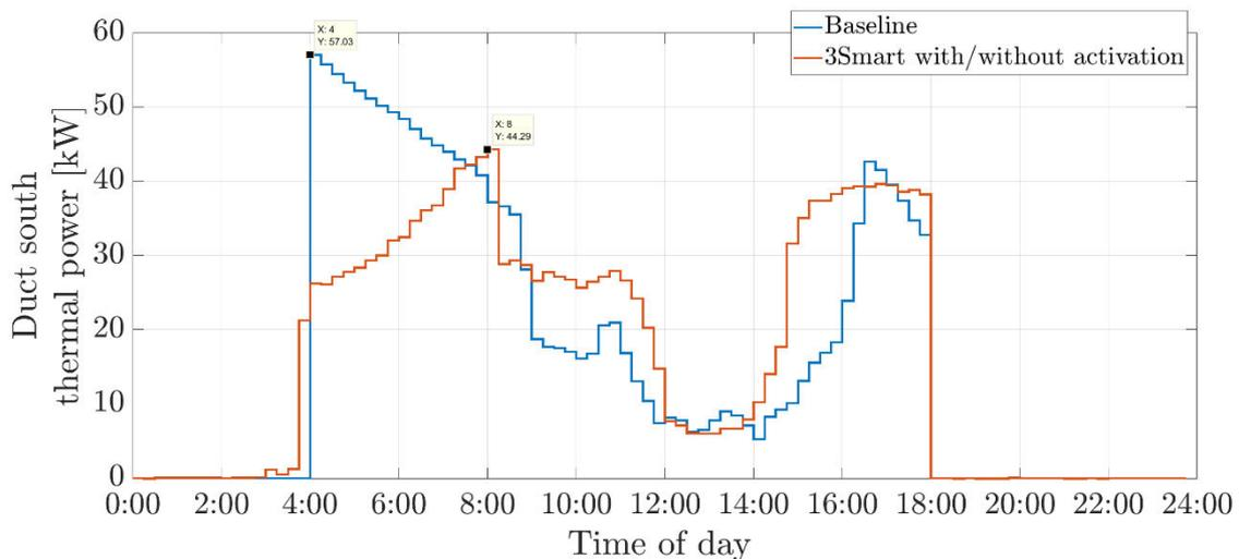
**Figure 3.30.** The overall heating energy consumption on duct south.
