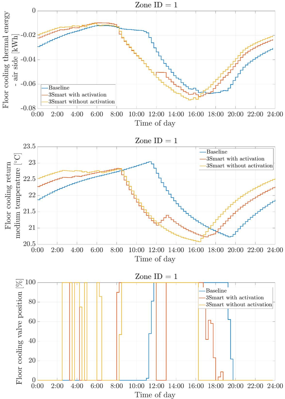
Figure 3.6. Cooling energy provided from the floor cooling element to room air. Return medium profile and valve opening.
