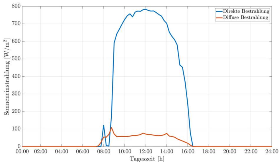
**Figure 2.2.** Direct (normal) and diffuse (horizontal) solar irradiance for a sunny day in November.
