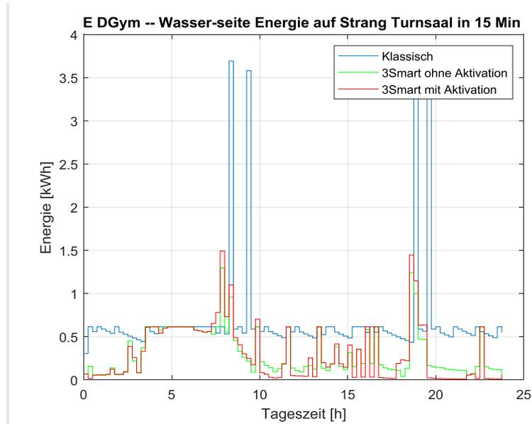
**Figure 2.47.** Consumed water-side energy on duct gym.
