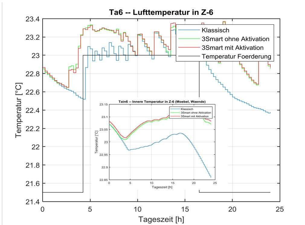
Figure 2.26. Temperature behaviour in Z-6. Small figure shows the behaviour of the inner room temperature state (representing walls and furniture).
