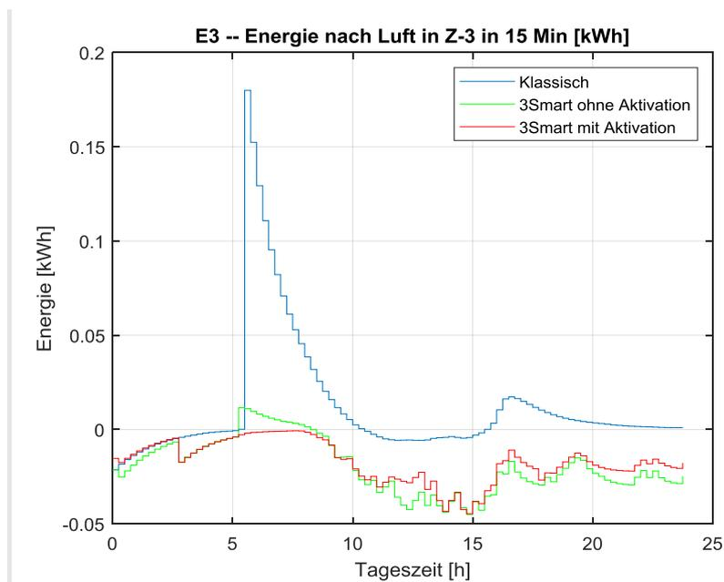
Figure 2.16. Energy provided to air in Z-3.
