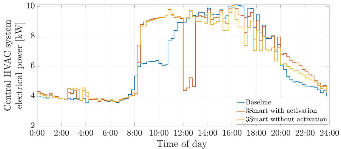
**Figure 3.10.** The overall electricity consumption on the central HVAC system level for the analysed day of operation in the retirement and care centre.
