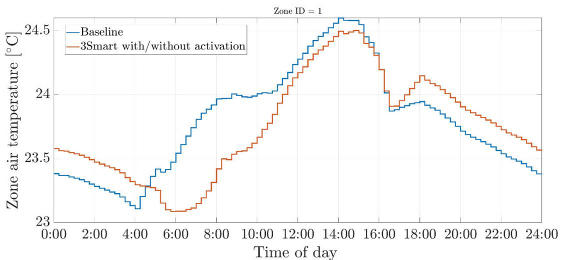
**Figure 3.18.** Temperature behaviour for one selected room in the retirement and care centre building within the analysed day.
