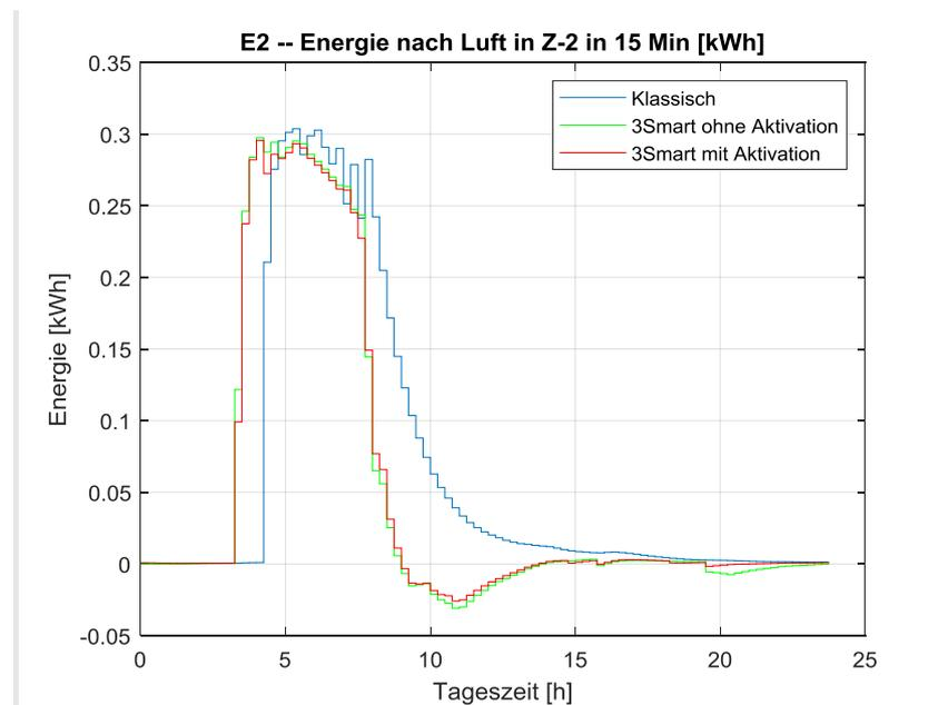
Figure 2.12. Energy to air in Z-2.
