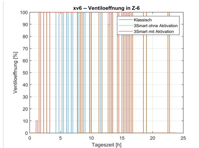
Figure 2.29. Valve opening in Z-6.
