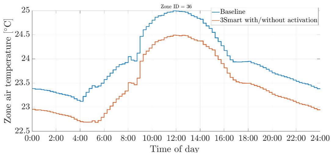
**Figure 3.22.** Temperature behaviour for a room in the retirement and care centre building within the analysed day.
