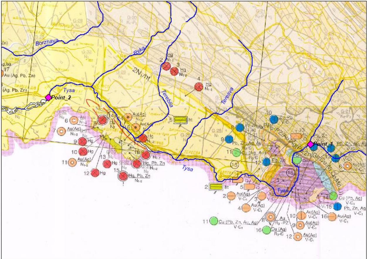
Fig.42: Metallogenic map of the area of work (original scale 1: 500,000; 2003). Circles indicate the location of geochemical anomalies, their elements and the index of the rocks in which they are identified (denominator)
