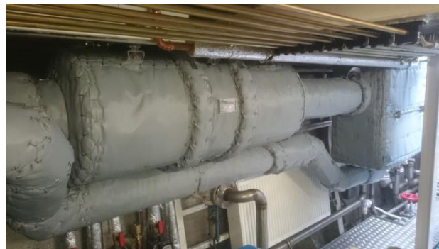
Figure 3: SCR and DPF on board of the MAX PRÜSS Source: www.wochender-umwelt.de
