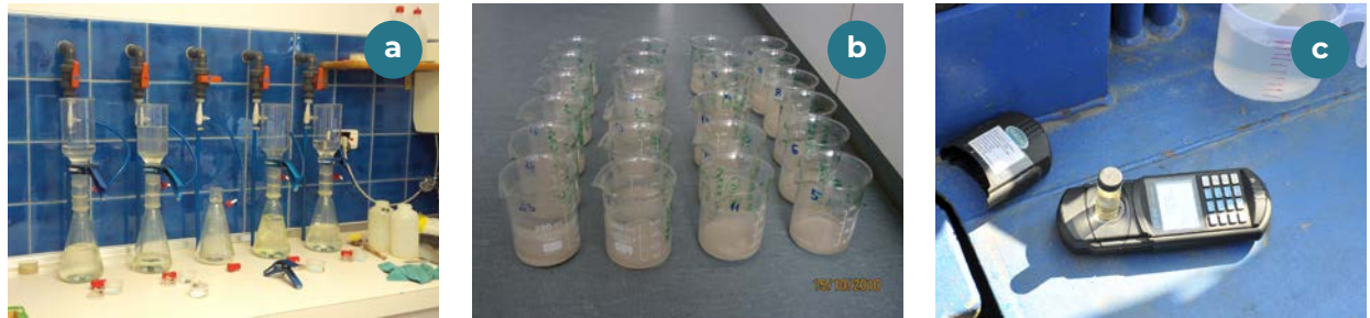
Figure 14: Methods to determine SSC: (a) filtering method, (b) evaporation method and (c) turbidity method (from the DanubeSediment report "Sediment Monitoring in the Danube River")
