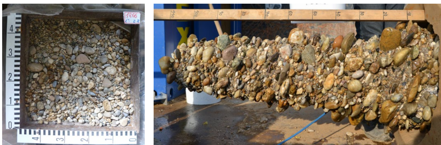
Figure 12: Volumetric bed material sample (left, photo: ©WRI) and freeze core sample (right, photo: ©IWA/BOKU).
