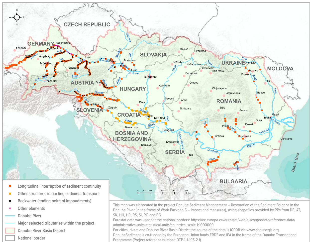
Figure 3: Spatial distribution of longitudinal sediment continuity interruptions on the Danube River and major tributaries selected in the project (from the DanubeSediment report "Interactions of Key Drivers and Pressures on the Morphodynamics of the Danube").
