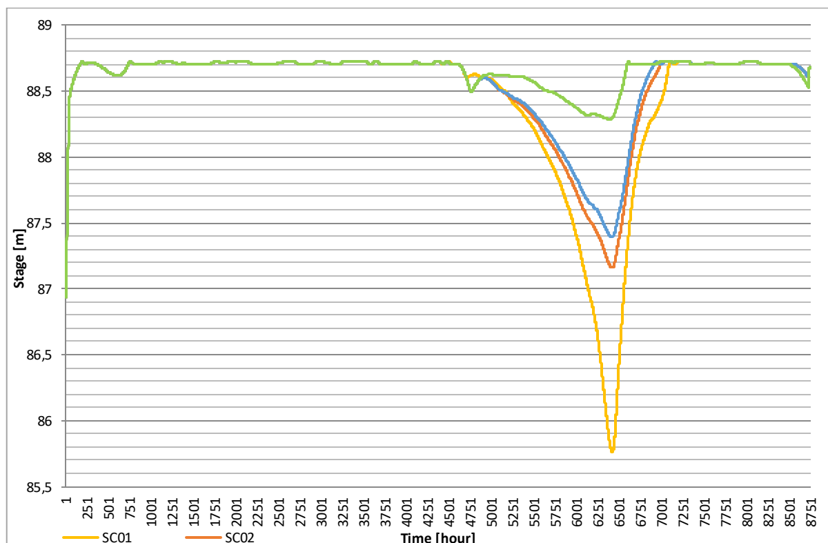
Figure VI.5: Water level at headwater of the Kisköre barrage
