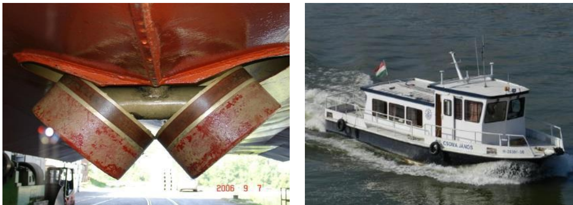
Figure 3.5: Head of multibeam echo sounder (left), Multibeam survey vessel (right) used for riverbed topography measurements in Hungary (Source: Middle-Danube-Valley Water Directorate)
