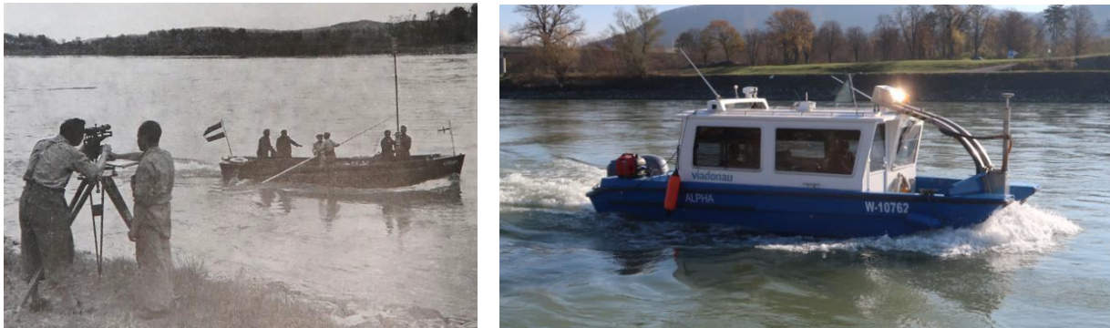
Figure 3.1: Left picture: Bathymetry measurement in the past, using a “Doppelbild Tachygraph” (Embacher, 1969); right picture: viadonau’s multi-beam bathymetry vessel during (photo: Philipp Gmeiner /BOKU)
