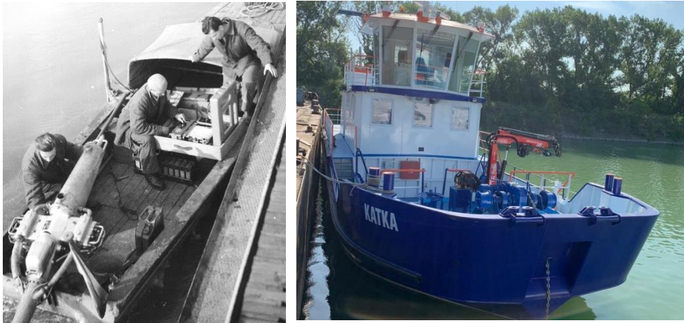
Figure 3.3: Left: Bathymetry measurement performed by VÚVH using EchoLog during a surveying campaign in the past, photo: VÚVH; Right: using an multi-beam vessel – present; photo: SWME
