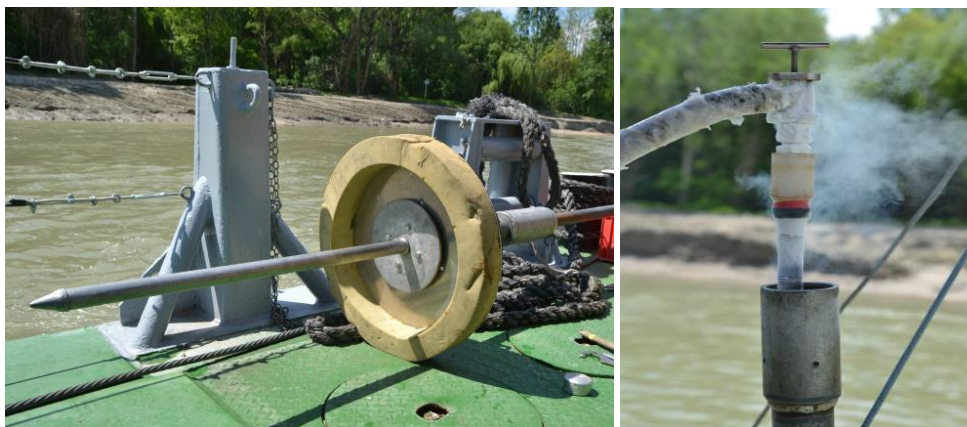
Figure 3.10: Left picture: Steel pipe and panel of a combi-corer used for freeze-core sampling; Right picture: Freezing procedure with liquid Nitrogen (photos: Sebastian Pessenlehner / BOKU)
