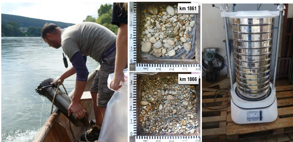
Figure 3.14: Volumetric sediment sampling and grain-size distribution analysis using a sieve shaker in the laboratory of VÚVH (photo: Holubová, Petrisko - VÚVH)
