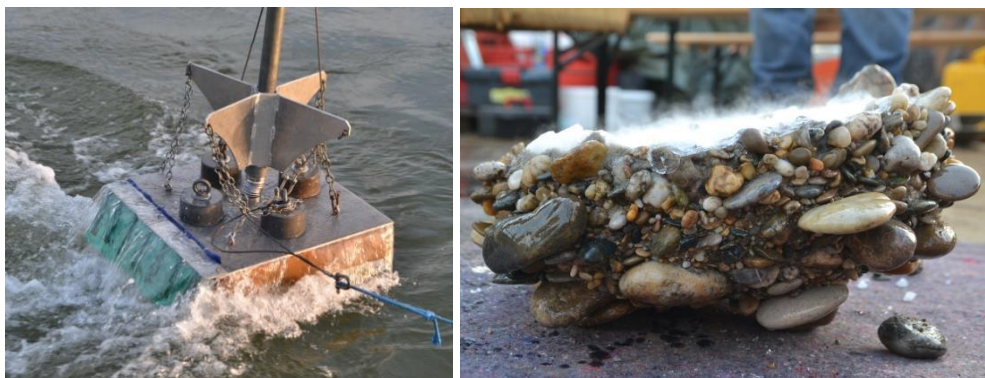
Figure 3.12: Left picture: Freeze-panel sampling; Right picture: A freeze panel (photos: Sebastian Pessenlehner / BOKU)
