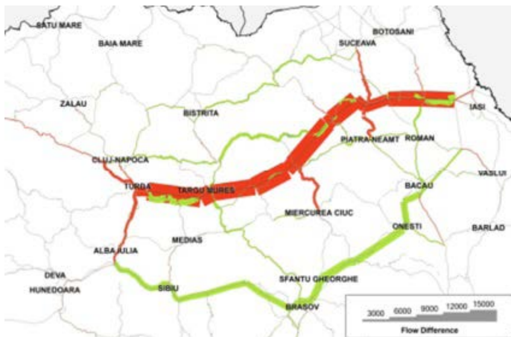
Fig. 3. - Predicted traffic flow changes after the finalization of the planned Tg. Mureş-Iaşi-Ungheni (A8) highway. Source: General Transport Master Plan of Romania.
