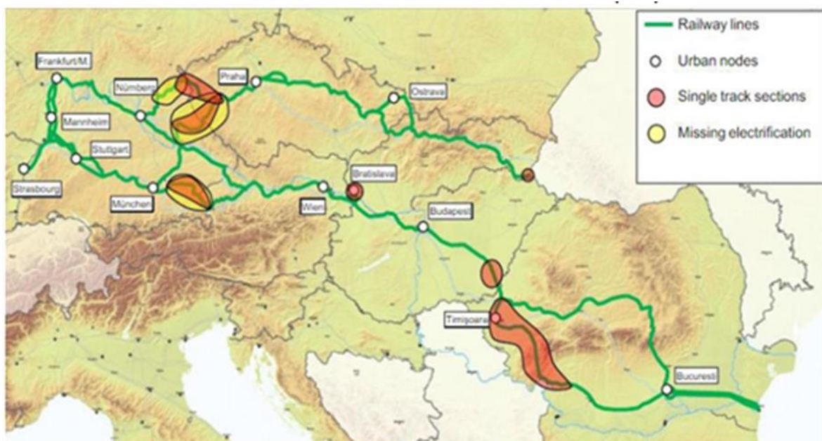
Figure 7 Single and non-electrified railway sections in DBS Gateway Region
