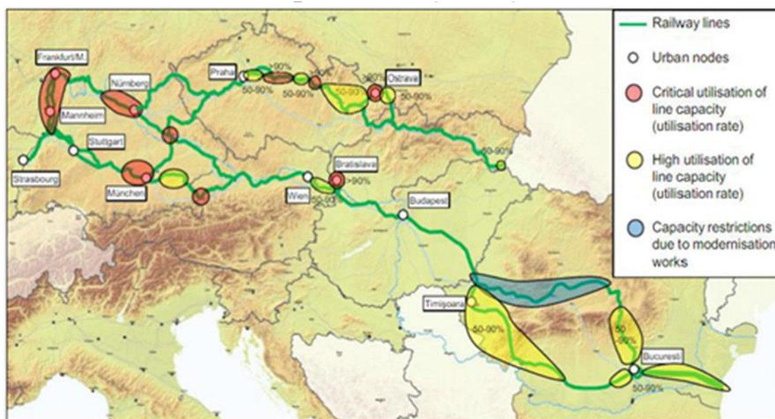
Figure 9 Railway capacity issues in DBS Gateway Region
