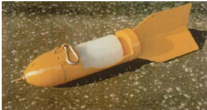
a) WRI sampler for depth-integrating sampling
