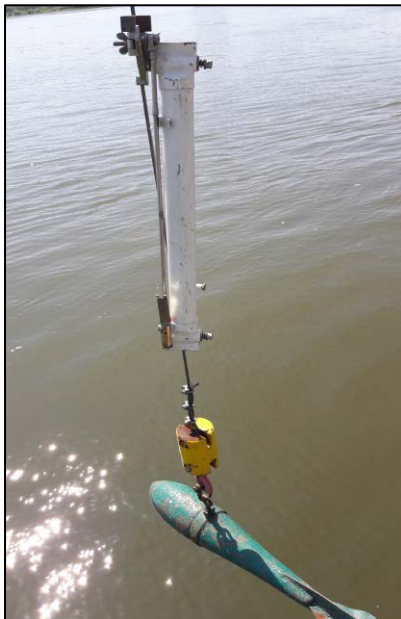
Figure 20 Suspended sediment samplers by the Romanian (left) and Bulgarian measurement teams
