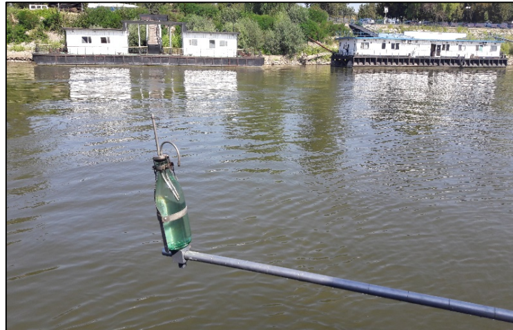
Figure 20 Suspended sediment samplers by the Romanian (left) and Bulgarian measurement teams
