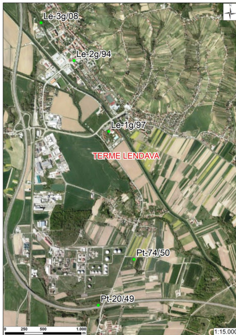
Fig. 36: Location of geothermal wells in Lendava. All five wells tap the Mura formation aquifer but Le-1g, Pt-20 and Pt-74 are used by Terme Lendava while Le-2g in and Le-3g form a geothermal doublet of the Petrol Geoterm Co.
