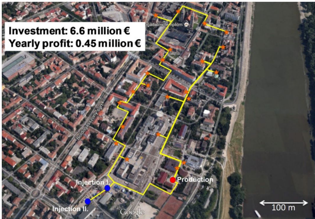
Fig. 25: Geothermal cascade system in Downtown with heat centers marked with orange stars
