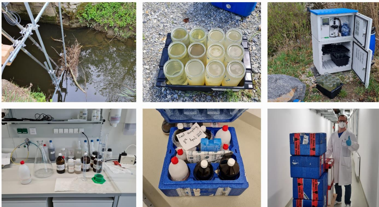
Figure 2: After each high-flow event the station had to be cleaned, samples picked up and mixed to form composite-samples, then distributed to the different lab bottles and then send to the laboratory for analysis.
