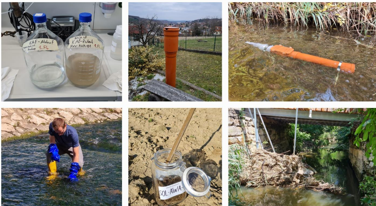
Figure 1: Compartments of the DHm 3 c monitoring campaign. Top: WWTP out- & inflow, amt. Station, Philipps-sampler. Bottom: low-flow grab sample, soil sample and online station after high-flow event
