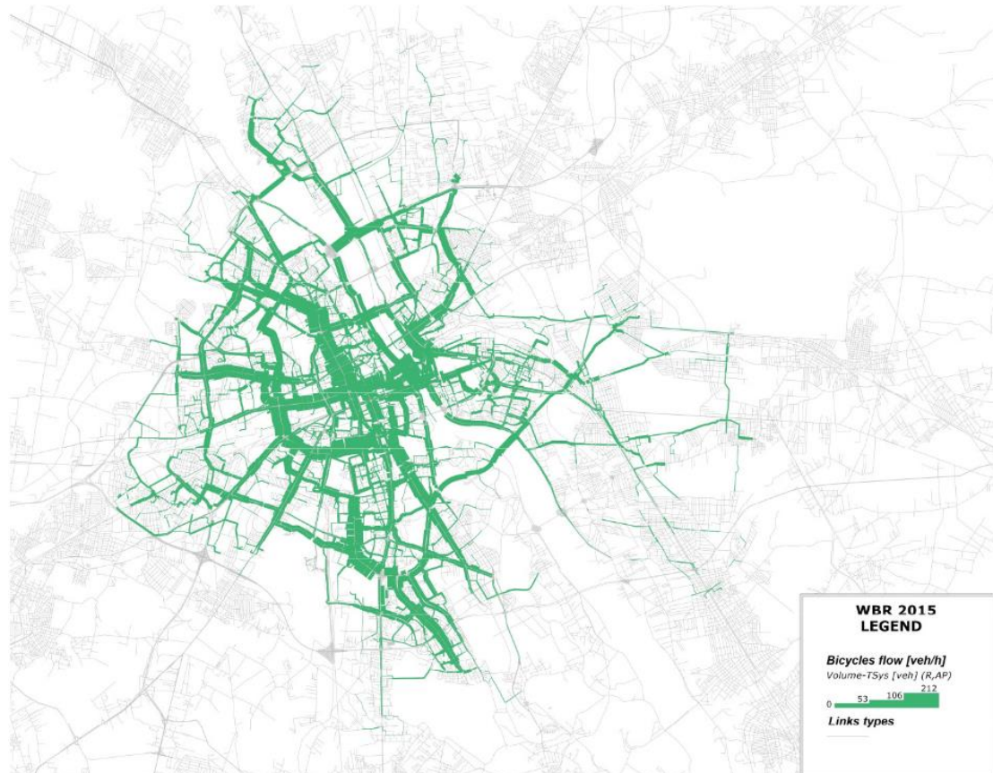
Figure 5. Bicycle trips distribution for 2015, morning peak. Source: developed using MTAW 2016 in VISUM. [46]
