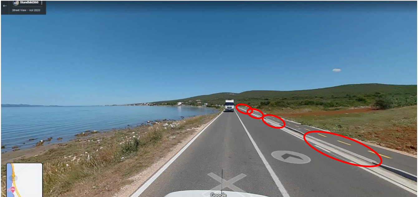
Figure 59. Croatia, Turanj: cycle track along the road is lowered every few meters due to the road entrances to the field. A few passes a week by cars should not be more important than continuous and safe cycling. Source: Google maps
