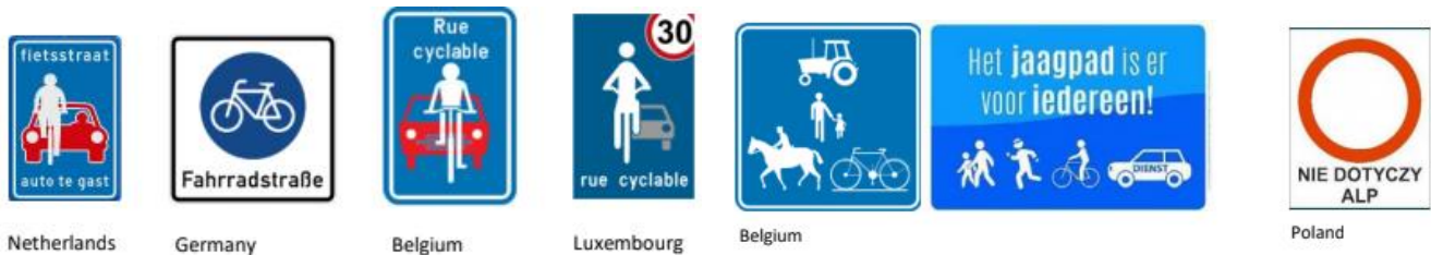
Figure 111. Examples of different road signs in use for a cycle street. Source: https://drive.google.com/drive/u/1/folders/1Rd-PtDgTpElgthQBKf8HiaP9x4jt7AKd
