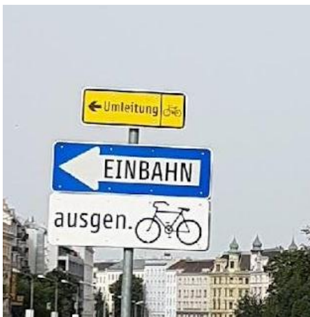
Figure 103. Austria: sign for the detour of the cycle track and exception of the one-way road (contra flow). Source: Sindikat biciklista
