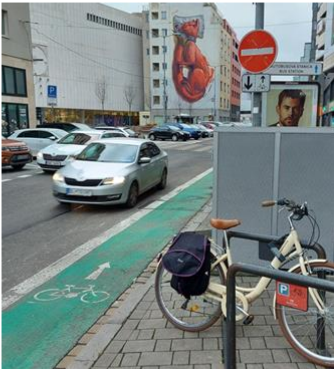
Figure 23. Example of contra flow advisory cycle lane from Slovakia. Source: DCP design standards, Peter Klučka
