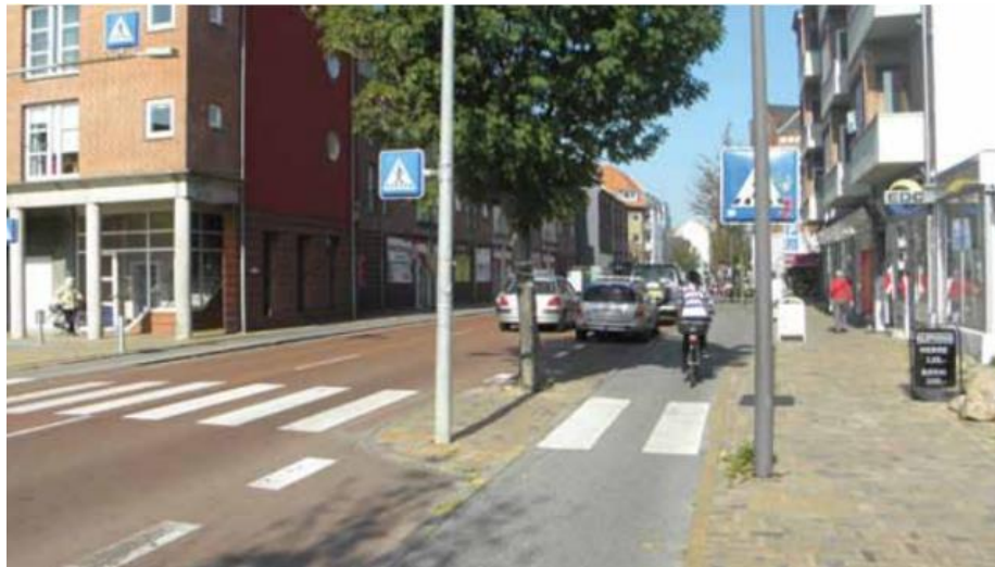
Figure 74. Safe crossing for pedestrians across the cycle track. [1]
