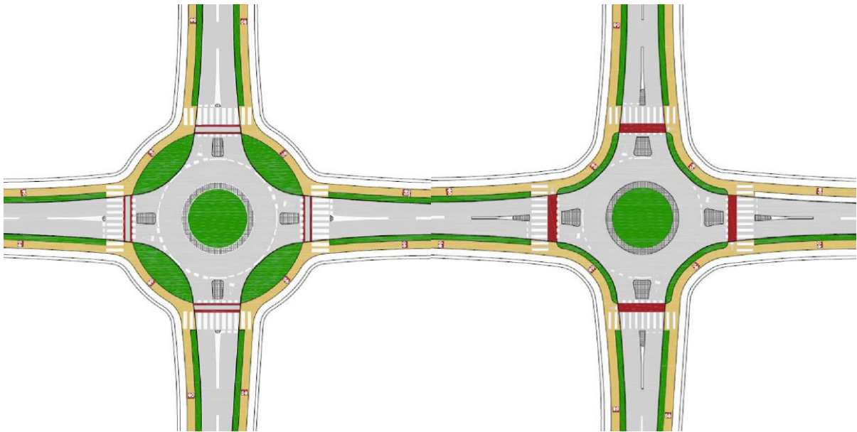
Figure 55. Course of the cycle track at the roundabout. [29]
