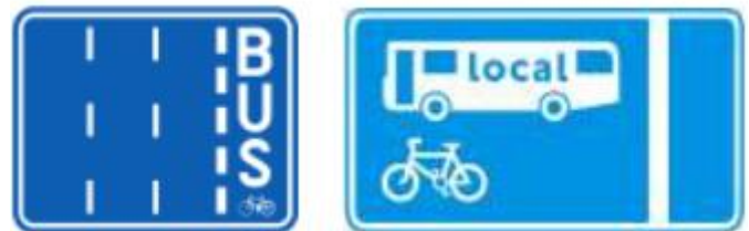
Figure 133. Signage for shared bus-bike lanes in Belgium and England. Source: PRESTO Factsheet on bicycles and buses.
