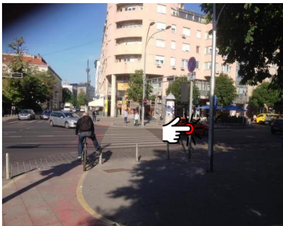
Figure 70. Example of a pushbutton for cyclist and pedestrians which is 4 m away of the cycle track crossing. Source: Sindikat biciklista
