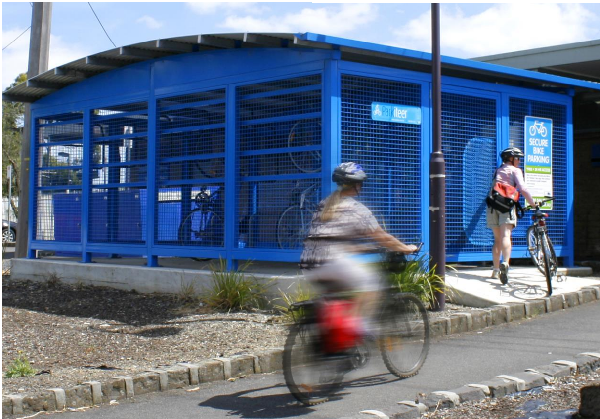
Figure 94. Collective bicycle lockers (bicycle cages). Source: TIDE Guidelines for the implementation of Innovative bicycle parking scheme
