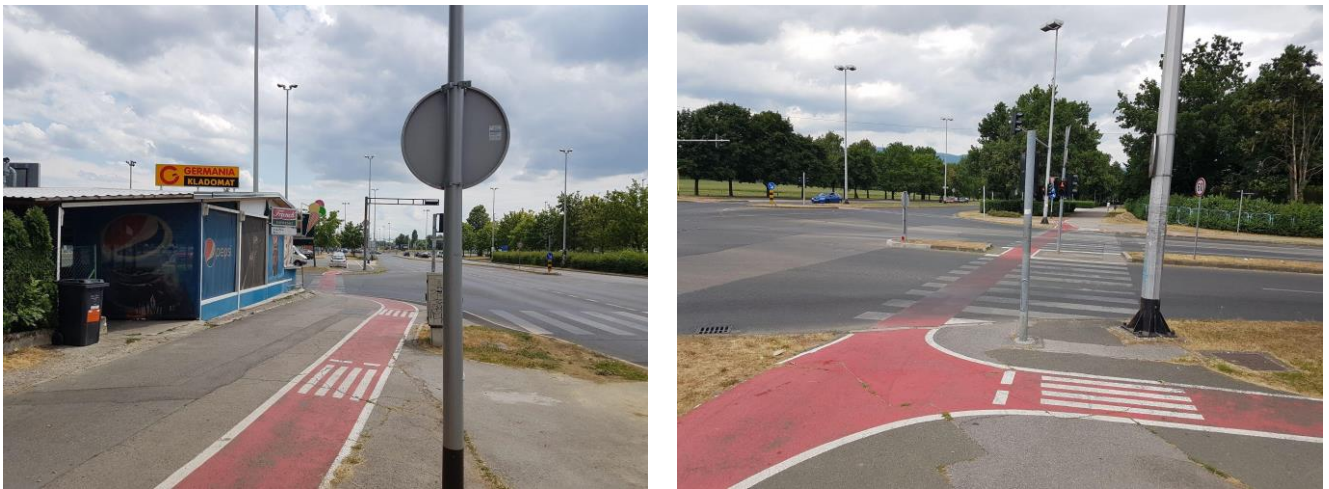
Figure 73. Pedestrian crossings over cycle tracks in Croatia where there is no marking guideline.
