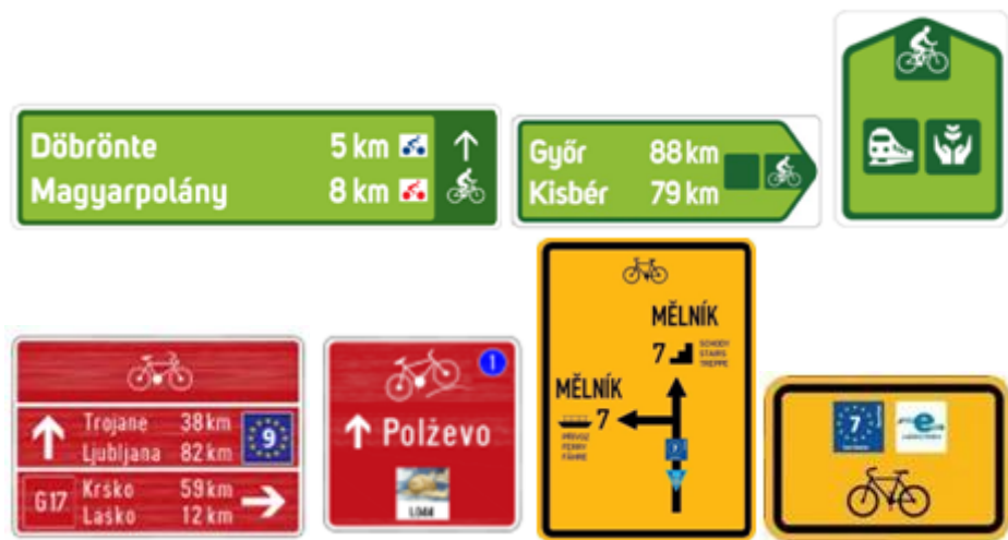
Figure 108. Signalization of cycle routes in national guidelines in Hungary, Slovenia and Czech Republic. Source: https://docs.google.com/document/d/1m1voy42N2J-drO3kVwdzh4w2jXFITRGo/edit#heading=h.19c6y18 , https://docs.google.com/document/d/1zUW72kLsL5tF3MkR19iw_uMcLU5_7D7h/edit
