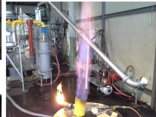
Burning of clean syngas which does not contain unwanted compounds like Furans, Dioxins, NO x , Tars or dust particles.
