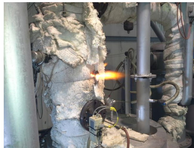
Testing in action: one of the prototype of catalyst – syngas broke through metal housing (left) and end result, clean syngas (down).
