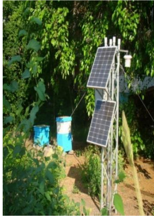
Meteorological station for measuring the microclimate in the bee colony and beyond
