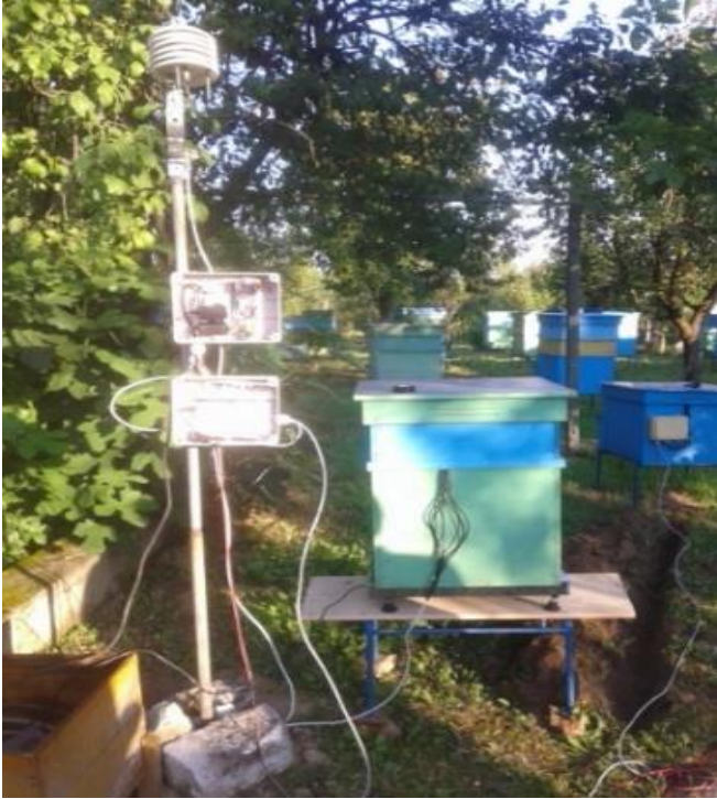
Meteorological station for measuring the microclimate in the bee colony and beyond
