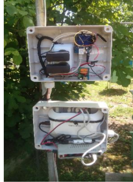
Meteorological station for measuring the microclimate in the bee colony and beyond
