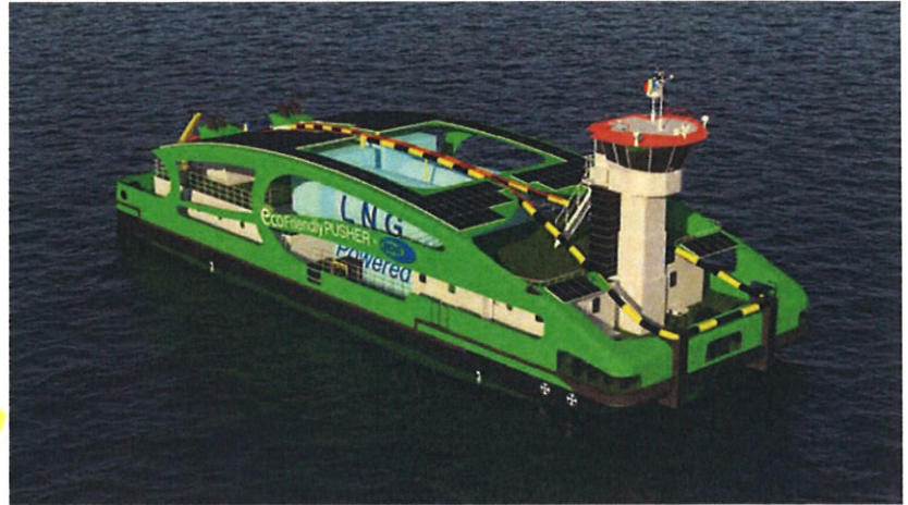
Rated more than 4,100kW, the proposed LNG inland pusher would be one of the most powerful vessels of its type on the Danube River
