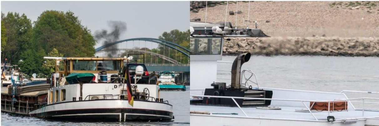
Figure 16: Pictures of exhaust plumes (left: engine reversing, right: typical appearance at steady state operation)
