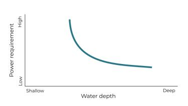
The relationships between required power, velocity of the ship and water depth are the main basis for EEN. This principle can be used to reduce energy consumption. The three most important facts are:
