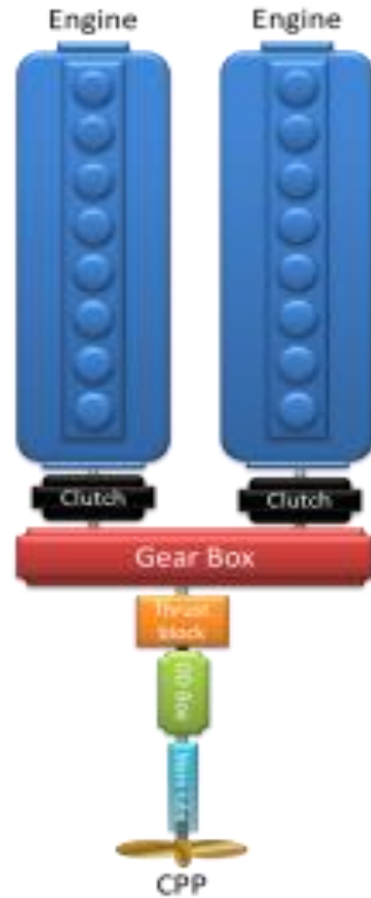
Two engines – one shaft
