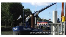
Vessel type: working boat ENI: 2325374 Vessel size: 37.58 m × 9.12 m (L × W) Propulsion: 2 × Vink - MX 11 – 240 kW
