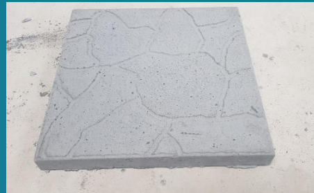
Tested concrete pavement made with waste sand.
