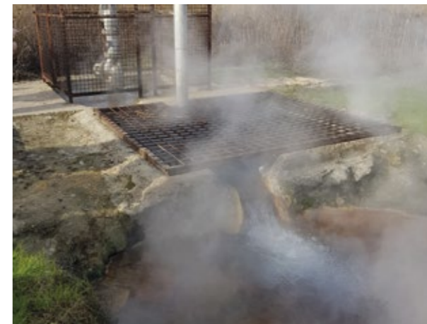
BB-2 well, an old hydrocarbon well drilled in the 1970's discovered thermal water with outflow temperature of 78 °C and 35,5 l/s, which was the first proof of existing rich geothermal resources nearby Bogatic
