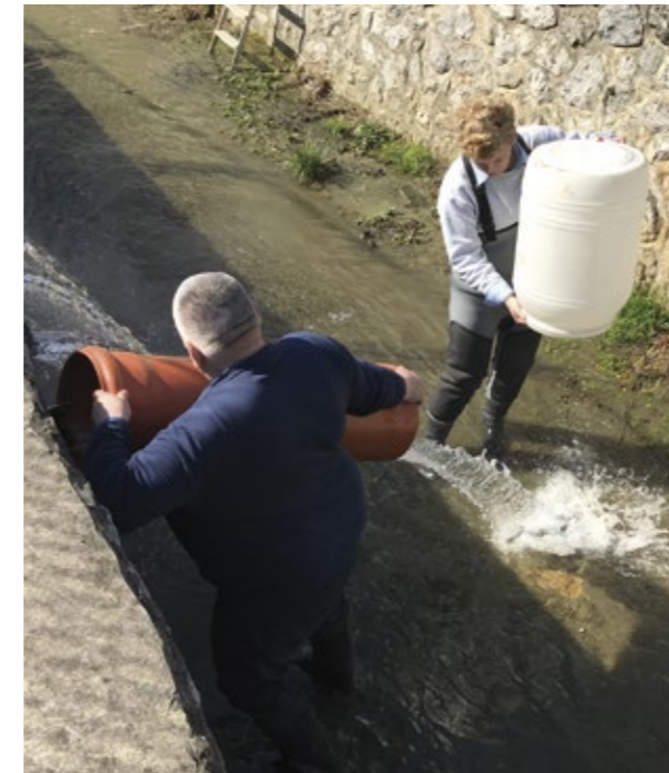
The yield measurements of the Jakobljeva kupelj spring (photo by D. Šolaja)
