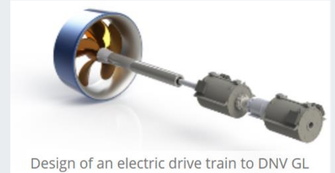
Inland Vessels with serielle and parallel Hybrid
