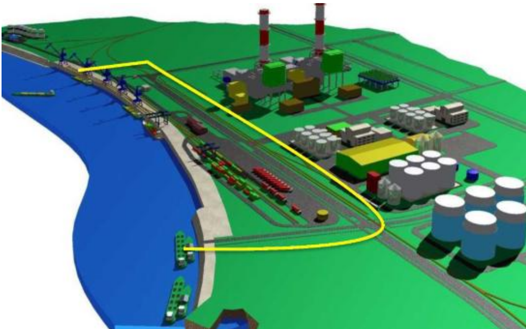
Figure 70: Layout of the future intermodal facility in the Port of Slavonski Brod
