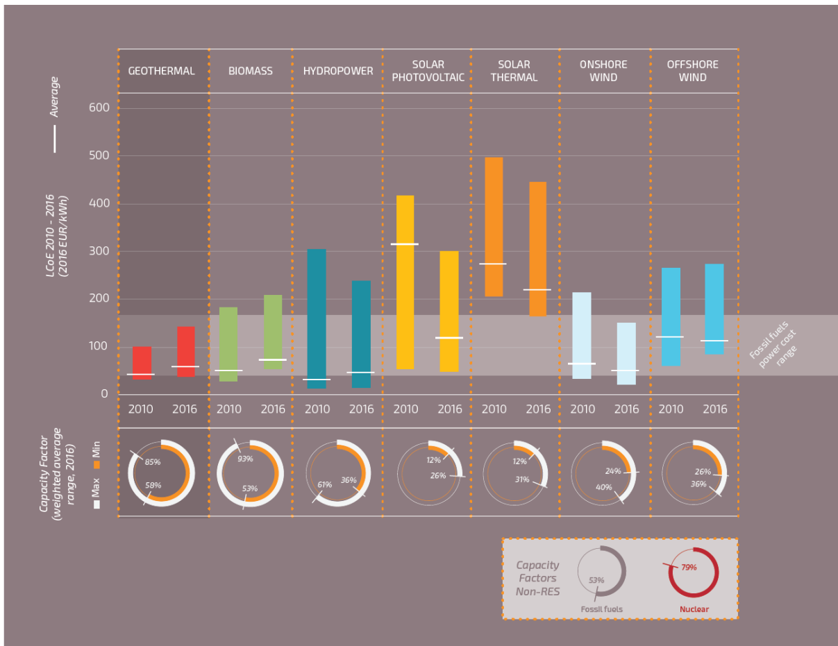
Figure 4: Comparison of capacity factors and LCoE of various renewable. From: Renewables 2017 Global Status Report, REN 21, EUROSTAT, IRENA 2017)
